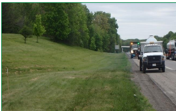
Photograph 36. A spray truck driving 9 miles per hour, making applications with a 22-foot nozzle, can treat 24.47 acres per hour, compared to mowing at 3.86 acres per hour. Only 917 acres per year needs to be managed with the spray truck to realize a return on investment by labor savings in reduced mowing requirements.
