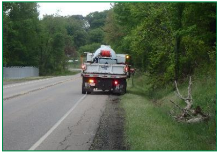
Photograph 20. Spray truck making a 10-foot-wide broadcast application along a typical two-lane highway.
