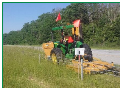
Photograph 13. Tractor pulling rear-mounted mower deck to clear overgrown vegetation between cable rail and shoulder.
