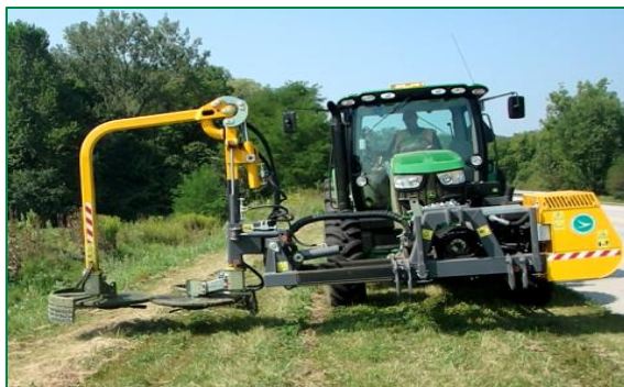
Photograph 4. U.S. Ditcher Inc. GM-60 Spider Guardrail Mower mounted on John Deere 6115 R Tractor
