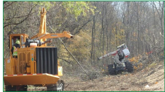
Photograph 109. The whole tree chipper is driven on tracks, has a cab, and a grapple arm to load chipper feed. This equipment can do the job of several pieces of equipment.
