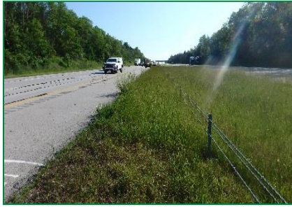
Photograph 15. This picture shows significant grass height differences between plots treated with PGR in the foreground and mow-only plots in the background.
