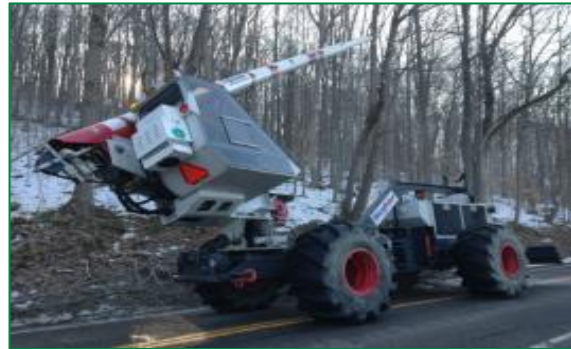
Photograph 95. All-terrain tree trimmer removing branches overhanging the road.
