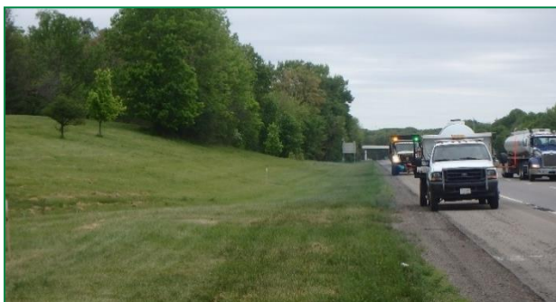
Photograph 7. Spray truck making broadcast herbicide application with a 22-foot-wide spray nozzle.
