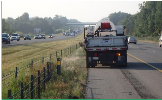
Photograph 6. Production efficiency of a spray truck making herbicide applications can provide labor savings of $633.54 per mile per year when compared to string trimming the mile four times per year. In 13 miles of Zone One management, the cost of the equipment has been returned in labor savings.
