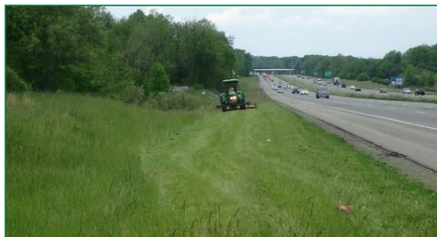
Photograph 8. Tractor mowing with a rear-mounted, hitch-drawn, 15-foot batwing mower deck.
