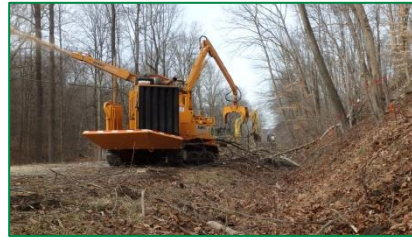
Photograph 106. Bandit 1850 chipper and excavator following all-terrain tree trimmer.
