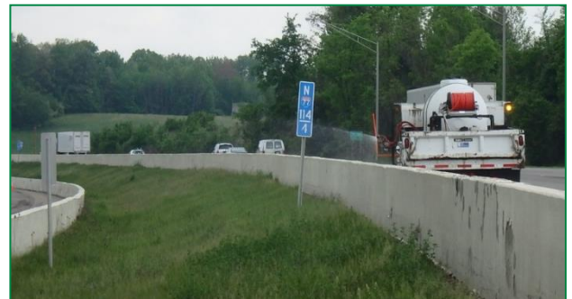
Photograph 29. Spray truck making a broadcast application over a barrier wall with a 22-foot spray pattern. Note the spray nozzle head height was adjusted to reach over the barrier wall.
