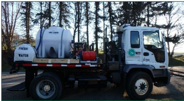
Photograph 18. Spray truck used in 2016 to make broadcast applications with boomless nozzle.
