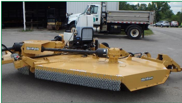
Photograph 23. Diamond WetBlade™ 15-foot batwing mower deck.
