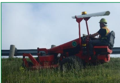
Photograph 33. Site 1 Treatment 1: Kut Kwick chariot-style riding mower with 72” rotary deck.
