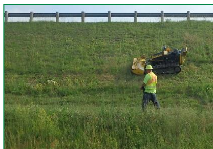
Photograph 34. Site 1 Treatment 2: Alamo Traxx™ RF Remote Control Mower with 51” front-mounted flail head.
