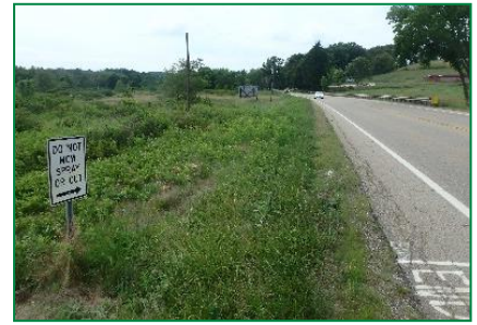
Photograph 22. A high percentage of broadleaf weeds are present in the mow-only plots. Weed height causes more of a concern to sight distance than turf height.
