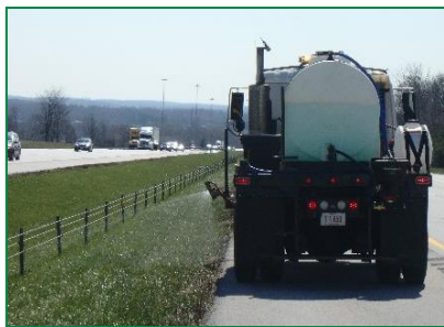
Photograph 12. Spray truck making PGR application in April 2016 with a 10-foot-wide spray nozzle pattern. The goal is to stop turf growth for 8 weeks.
