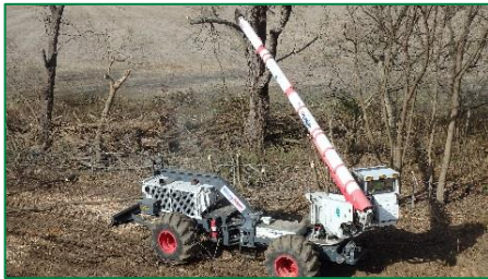
Photograph 99. ODOT employee trimming trees accessed off the road edge with an all-terrain tree trimmer.
