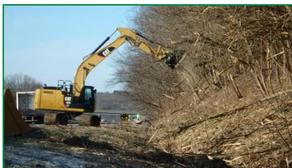
Photograph 110. The Brown Brontosaurus tree mulcher head on an excavator does the work of an entire tree crew with only one operator.
