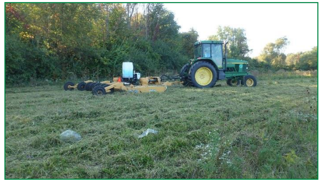
Photograph 24. Tractor with Diamond WetBlade™ mowing and applying broadleaf herbicide simultaneously.
