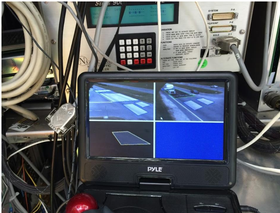
Figure 12. Video Detection Setup at the US460/Southgate Intersection
