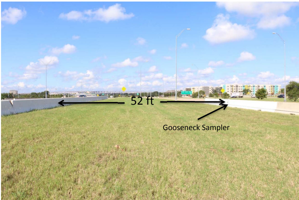
Figure 7.8 Photocatalytic sampling port (gooseneck) and proximity to roadway (goosenecks were placed on the northernmost barrier facing south)
