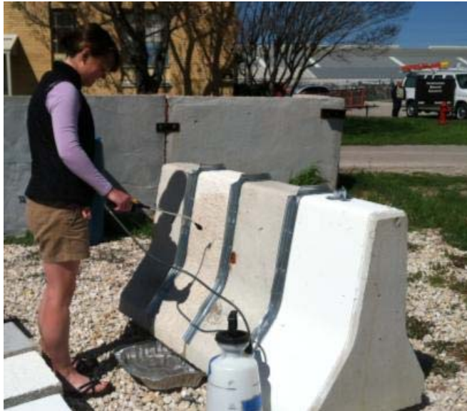
Figure 6.1 Concrete washing procedure
