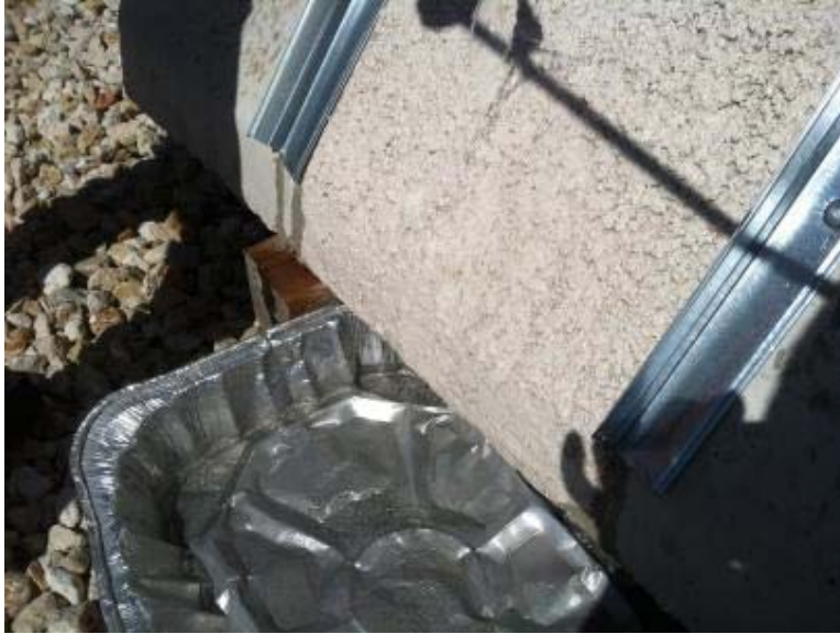
Figure 6.2 Water collection procedure for concrete specimens
