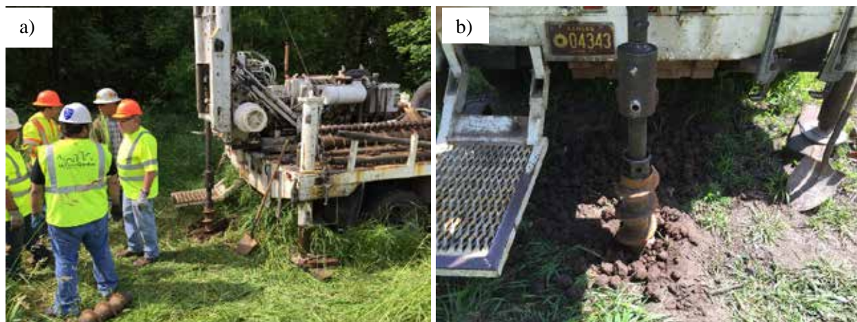
Figure 3.3: (a) Sample Drilling with the Drill Rig; (b) Close View of Drilling
