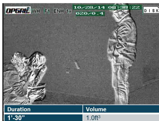
Figure 21 Successful Detection of Gas Leaks at 30 feet Distance
