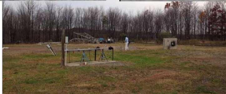
Figure 24 Successful Detection of Underground Gas Leaks at 50 feet Distance
