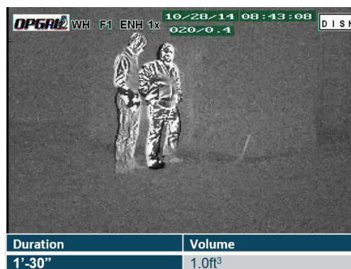
Figure 21 Successful Detection of Gas Leaks at 30 feet Distance
