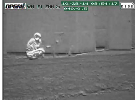
Figure 23 Successful Detection of Gas Leaks at 100 feet Distance
