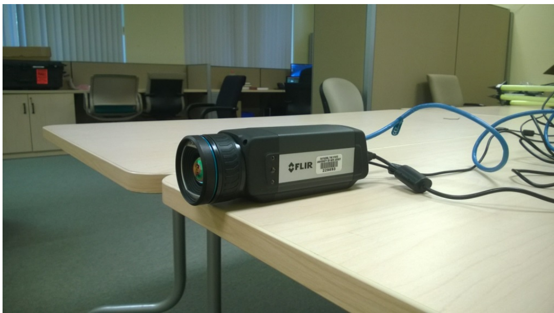
Figure 9 The FLIR Infrared Camera
