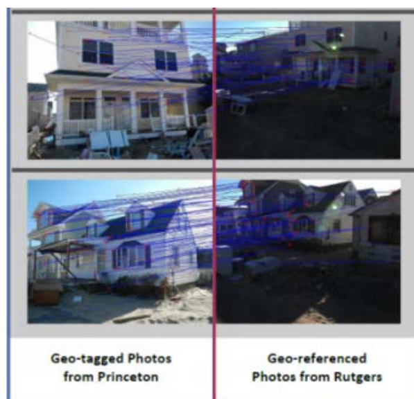
Figure 4. SIFT-based Matching between VGI photos and Mobile Lidar Imagery
