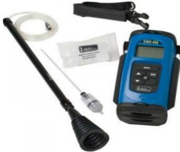
Figure 5 - Infrared Controlled Interference Polarization Spectrometer DP-IR, Heath Consultants Inc.
