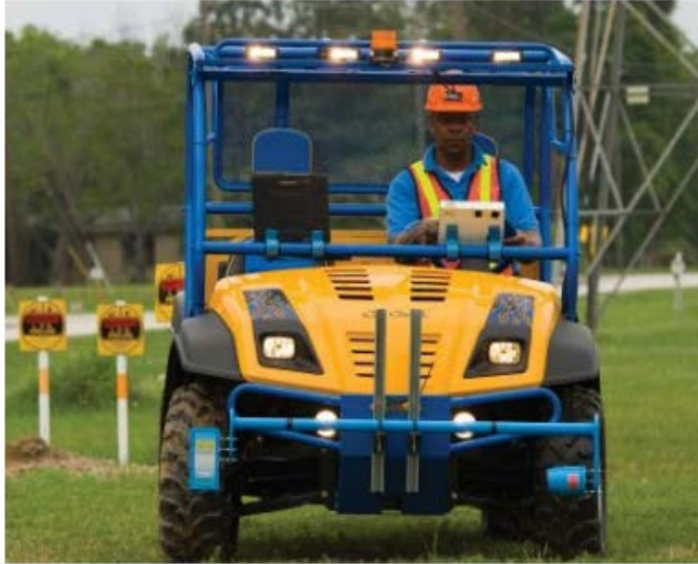
Figure 2. Optical Methane Detector (OMD) mounted on survey vehicle, by Heath Consultants Inc.
