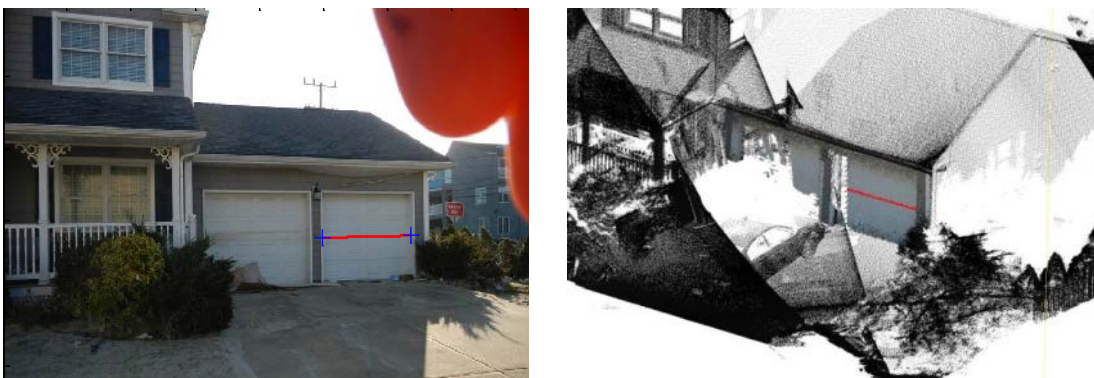
Figure 7. High Water Mark Measurement from VGI Images and Point Cloud Data
