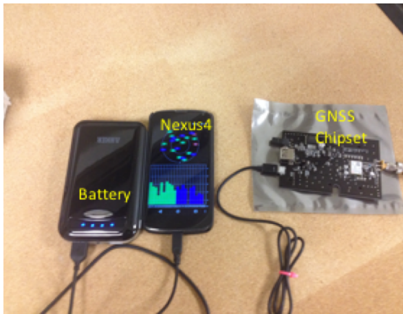
Figure 3: Nexus4 Smartphone with u-blox NEO-7P external GNSS receiver and external battery pack.
