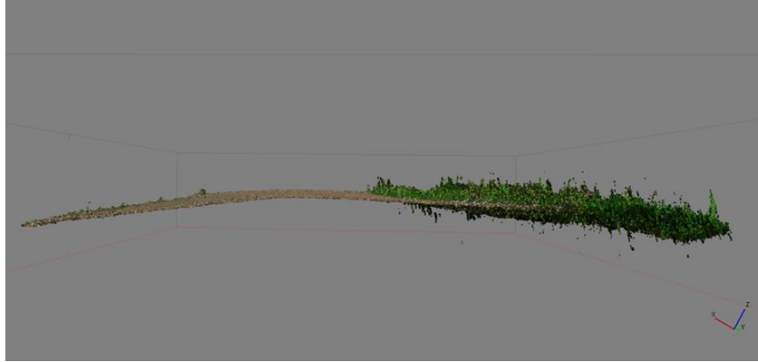
Figure 3-15: 3D point cloud on a section of unpaved road from the demonstration site illustrating the project team's capability to make crown measurements.
