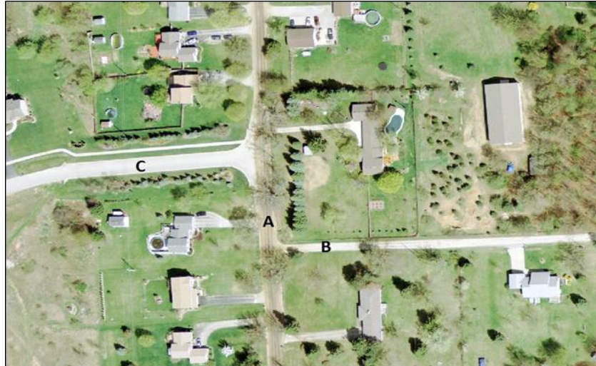
Figure 3-44: Example of RGB aerial photography being analyzed with image processing to map the location of unpaved vs. paved roads in SE Michigan as a mission planning input.
