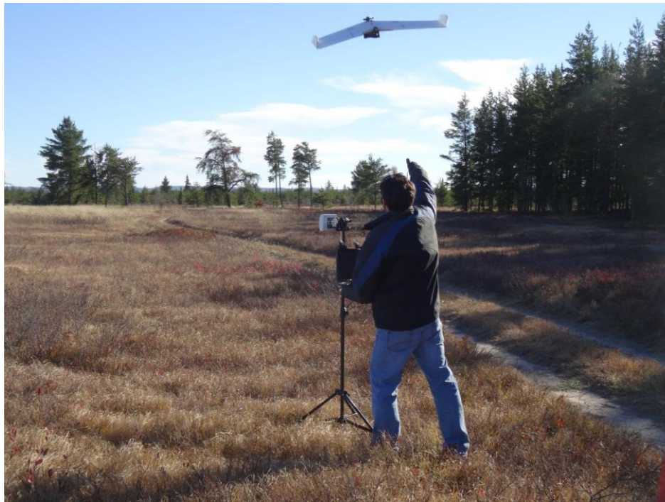
Figure 3-3: Lehmann LP-960 being hand launched and manually controlled.
