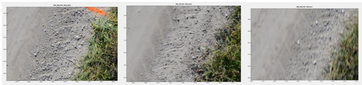
Figure 3-8: Sample images from Petersburg Rd collect, showing varying amounts of motion blur.
