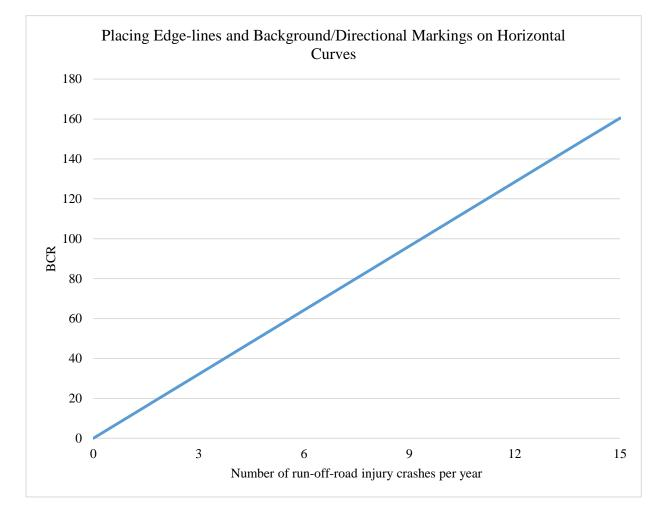
BCR for pavement marking of rural horizontal curves
