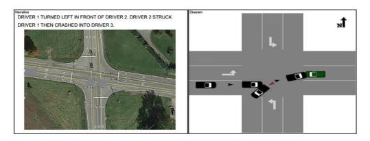
Figure 4.16 Example of crash type that can be avoided by providing left-turn offset
