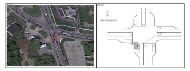
Figure 4.13 Example of improper left turn maneuver at skewed intersection which resulted to a crash
