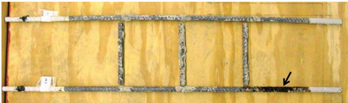
Figure 4.38 Corrosion in top mat of Specimen No. 28.
