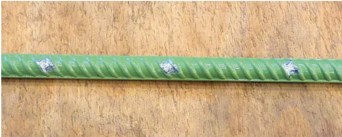
Figure 2.12 Damage introduced in epoxy coating (Lyrenmann, 2011).
