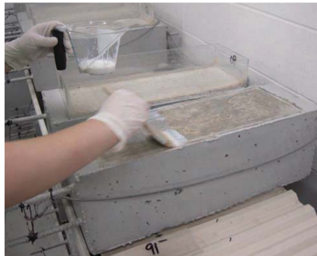
Figure 2.19 Applying deck sealer to uncracked control Specimen No. 91.
