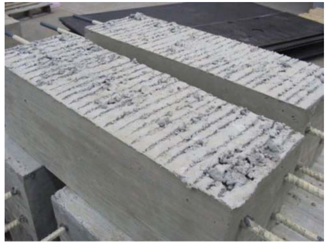
Figure 2.14 Specimens with surface tining (Lyrenmann, 2011).
