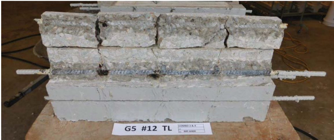
Figure 3.6 Steel-to-concrete interface at autopsy.
