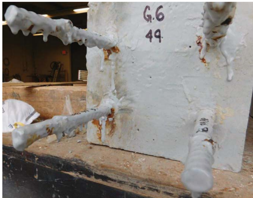
Figure 3.1 Corrosion of exposed steel.
