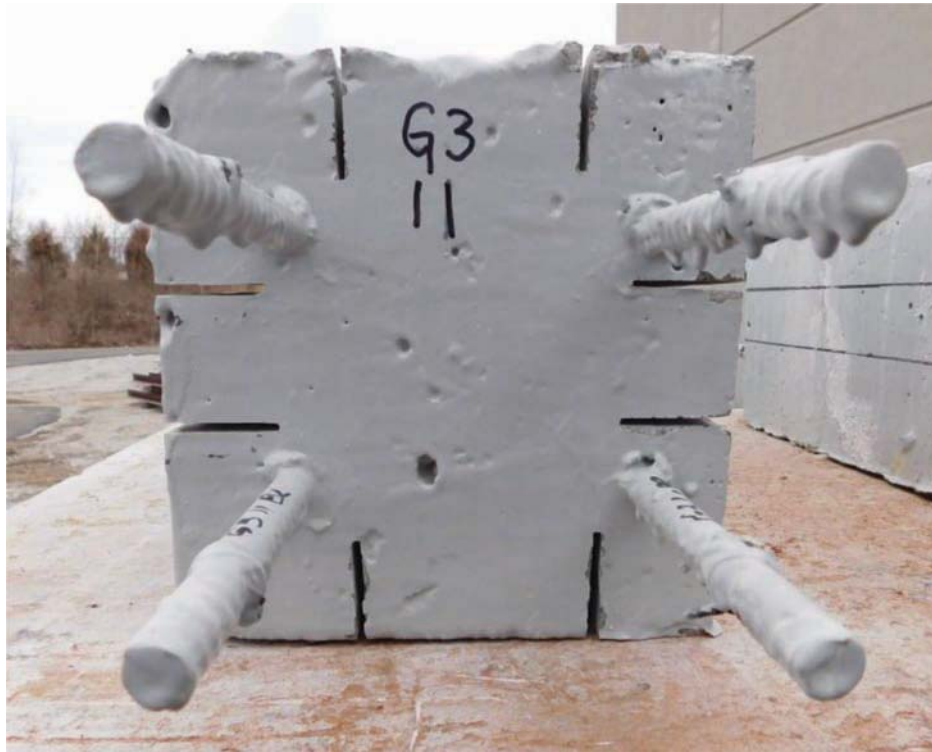
Figure 3.4 Specimen with completed cuts.
