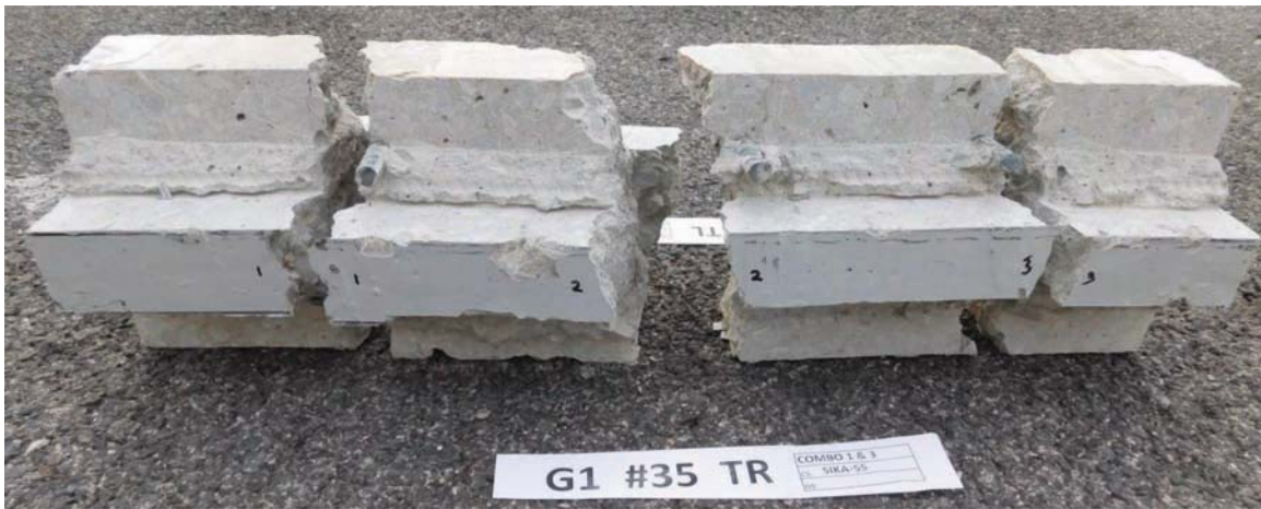
Figure 3.7 Specimen split at the cracks.
