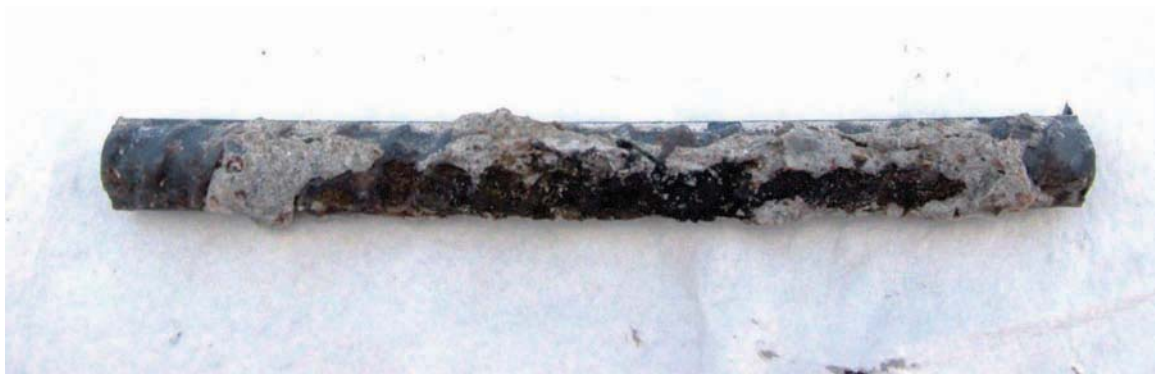
Figure 4.28 Specimen No. 14—close-up of front top transverse bar.
