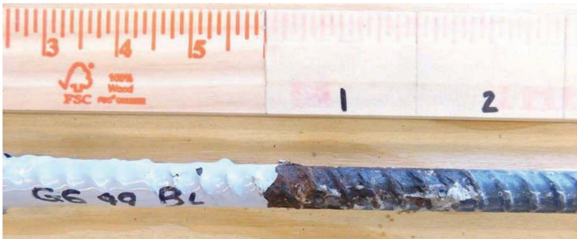
Figure 4.29 Specimen No. 49—corrosion on bottom left longitudinal bar.
