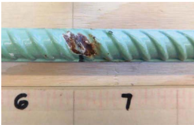
Figure 4.62 Specimen No. 33—close-up before epoxy removal on June 8, 2016.
