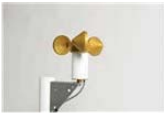
Figure 1. Mechanical Anemometer – Wind Speed Only.
