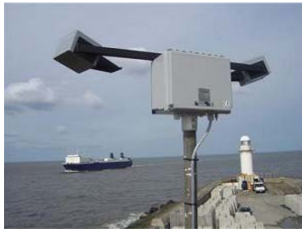
Figure 18. High Sierra Visibility Sensor – Model 5434-00.
