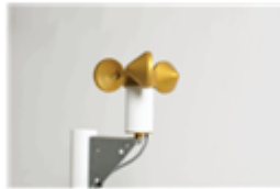
Mechanical Anemometer (Wind Speed Only)
