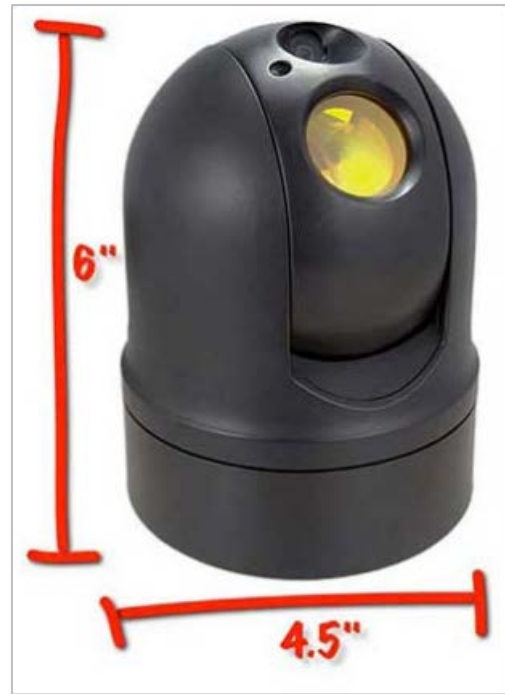
Figure 3 Thermal / Visible Video Camera Used for this Project
