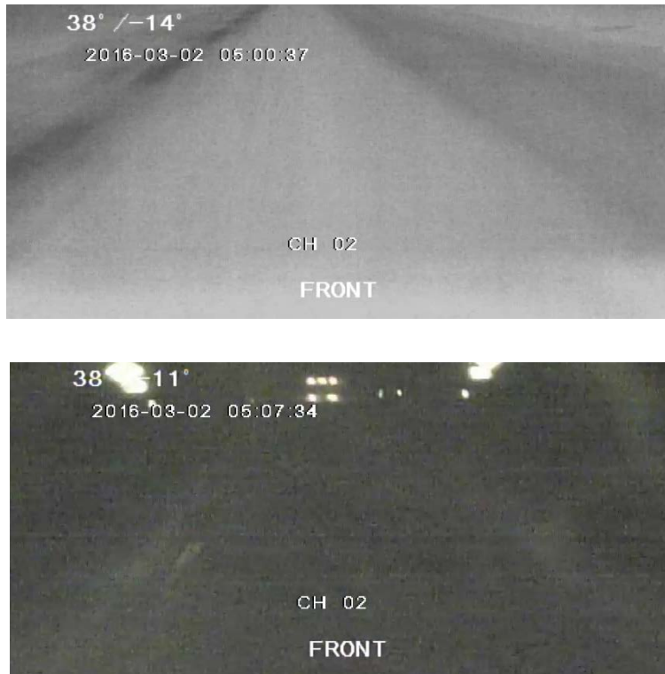
Figure 4 Thermal (top) and Visible (bottom) Imagery in Low-Light, Pre-Dawn Conditions
