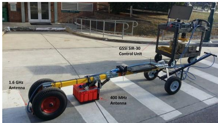
Fig. 12 GSSI SIR-30 dual-antenna installation
