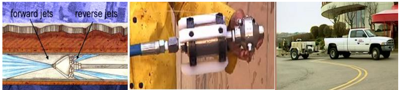
Figure 19 Cleaning a Trench Drain by a hydrojetter
