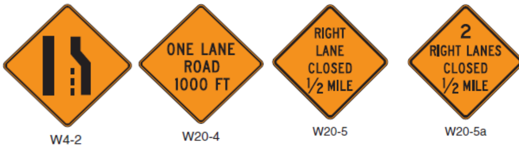
Figure 3-6. Example of Signs used to Indicate a Changed Roadway Configuration Involving a Lane Closure
