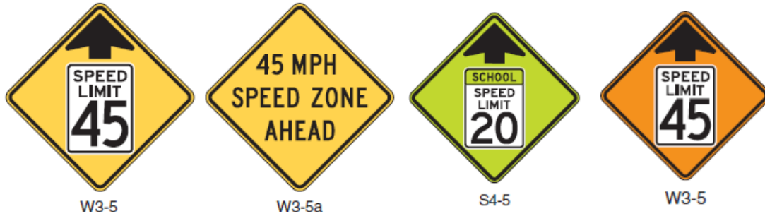
Figure 3-4. Example of Signs used to Indicate a Reduction in the Speed Limit Ahead for Various Types of Speed Zones
