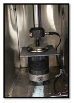
Figure 13 Sweep test compactor and compaction using the MTS: (a) Sweep test compactor and (b) compaction with MTS
