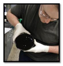
Figure 10 Binder application process: (a) pouring emulsion on the sample, and (b) spreading the binder by gravity & rotation
