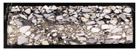
Figure 31 Cross sectional image of a double chip seal sampled in this study
