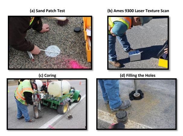
Figure 6 Procedure for taking cores from the field
