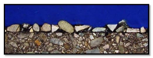
Figure 16 Desired cross section image
