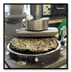
Figure 30 ASTM D7000 sweep test setup used in the current study
