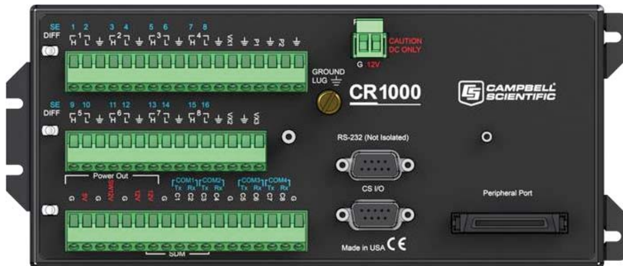
Figure 3.6: CR 1000 Data Acquisition System.
