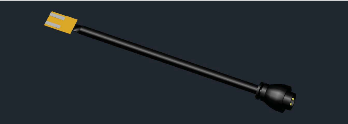
Figure 4.2 AutoCAD drawing for the Ice state and Presence Sensor Sensing Element and Connector.
