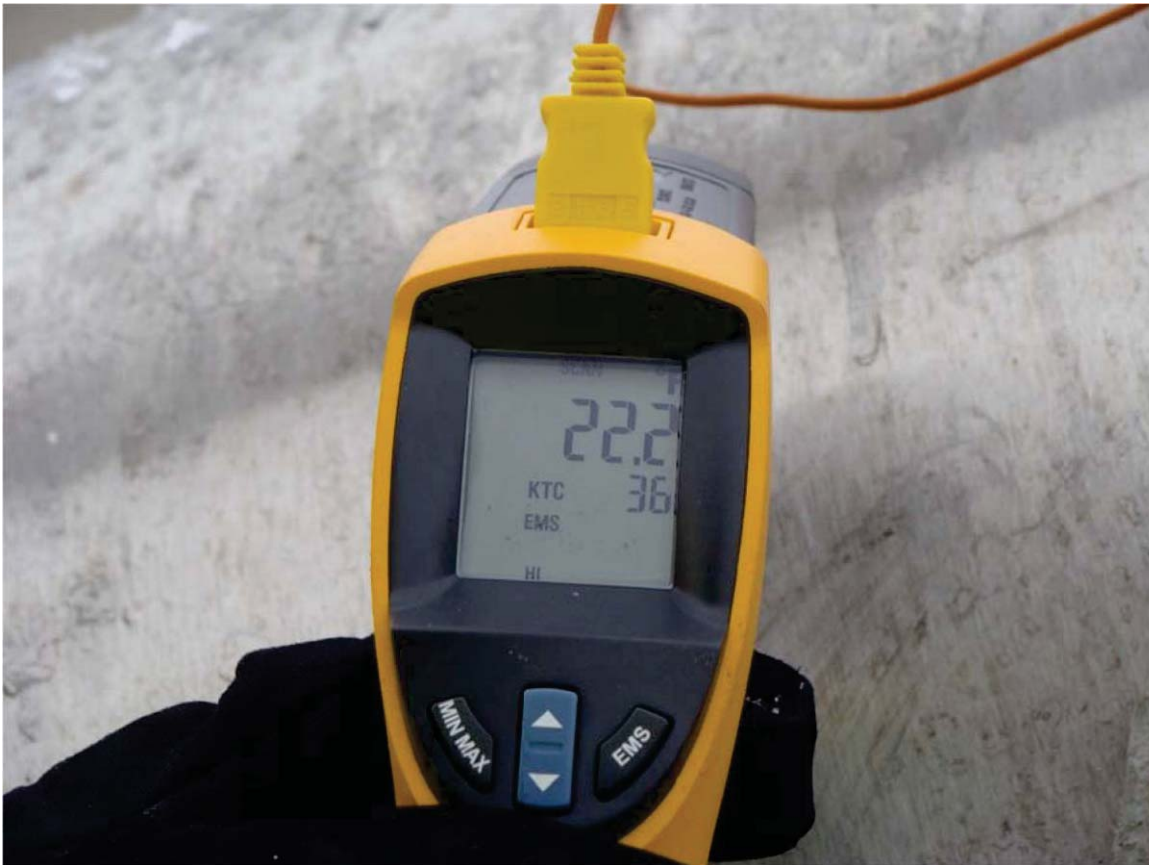
Figure 1.13: Thermocouple reading between ice and stay February 23, 2011
