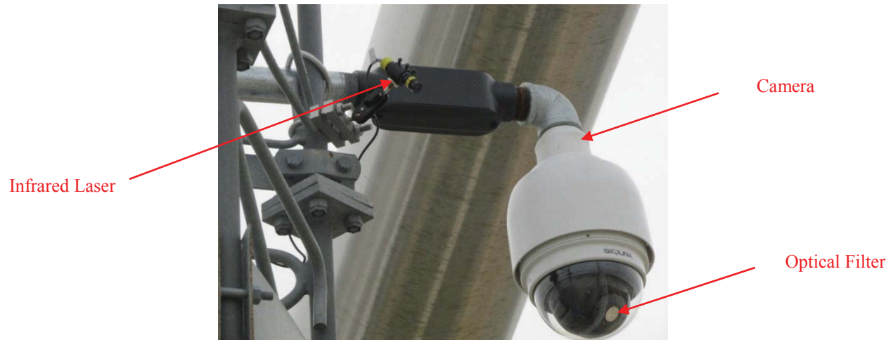
Figure 5.1 UT Optical Sensor Installation on VGCS Bridge.
