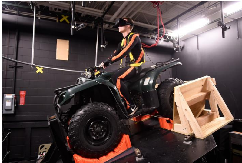
Figure 4.1 – ATV simulator. Note: This research assistant had his photo taken on the simulator without the helmet used by subjects during the study.
