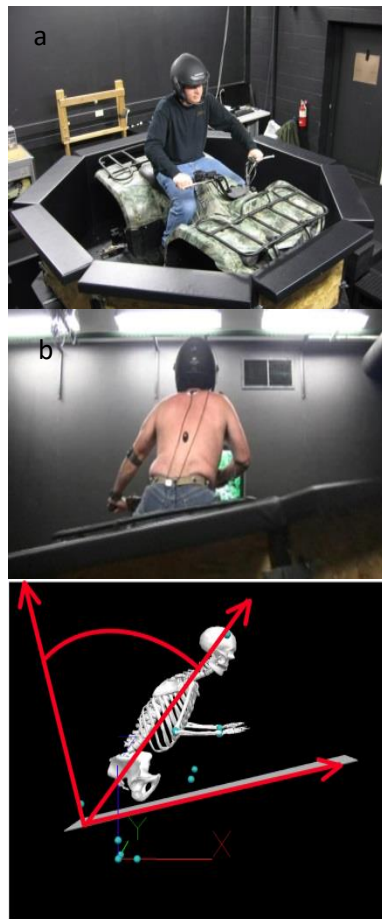
Figure 1.1 – Previous simulator: (a) original simulator used in pilot studies showing rider and safety features; (b) rider with motion-capture sensors and accelerometer instrumentation; (c) displayed model from data imported into 3D analysis software.
