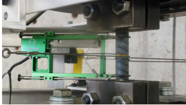
Figure 3.7: An extensometer attached on the reinforcing bar sample centered along the unbraced length
