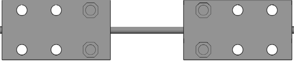
Figure 3.4: Schematic view of the clamps with a bar (side view)
