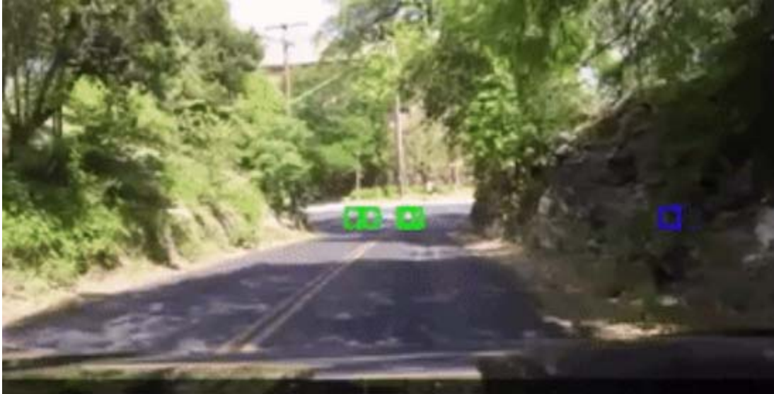
Figure 10.16: Blind intersection–DSRC detects approaching vehicle equipped with DSRC (blue square) and not visible to radar system. Radar false positives in green due to light reflex.
