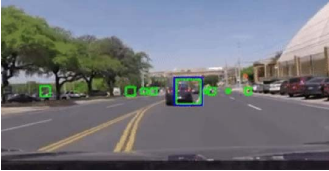
Figure 10.12: Accurate GPS data (blue square) sent through DSRC coincides with radar position detection (green square).
