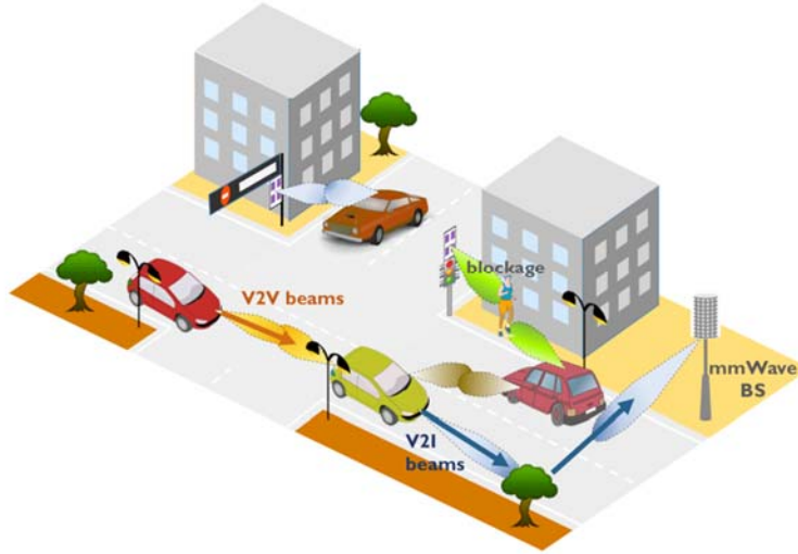
Figure 8.1: The conceptual figure of mmWave vehicular communications. Multiple mmWave transceivers are deployed on a vehicle to simultaneously establish V2V and V2I communication links.
