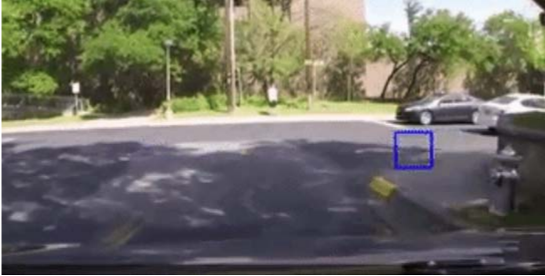
Figure 10.18: Blind intersection – DSRC detects approaching vehicle equipped with DSRC. Approaching vehicle is already in the field of vision of the driver but radar does not identify it.
