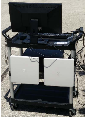
Figure 6.1: IEEE 802.11 joint radar and communications link setup for measurements. During measurements the antennas were not as close as in the configuration shown. The edges of these antennas were separated by a minimum of 0.5 m.
