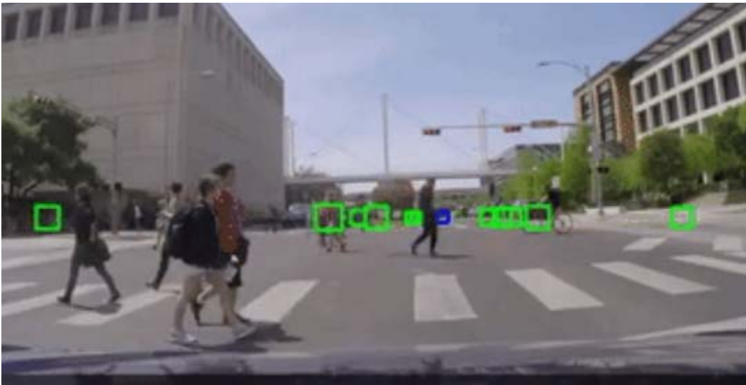
Figure 10.19: Pedestrian detection by radar–fails to detect pedestrians that are closer to the vehicle.
