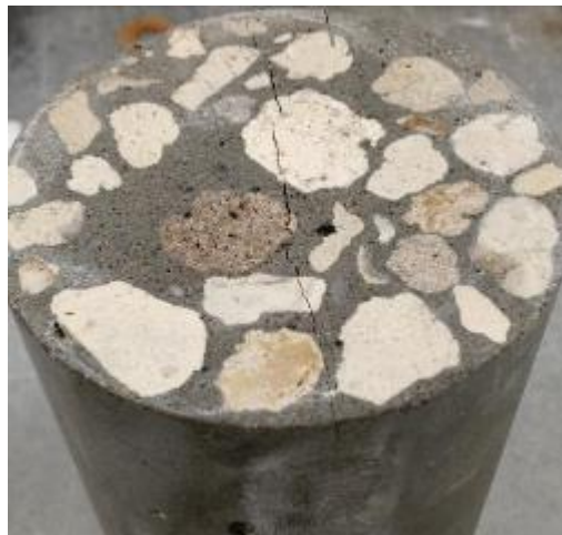
Figure 6-4. Fracture plane visible through the end of a failed splitting tensile specimen.
