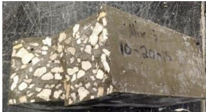
Figure 6-8. Typical flexure beam with failure through aggregates.
