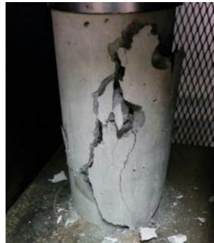
Figure 6-1. Concrete specimen loaded in compression to failure.
