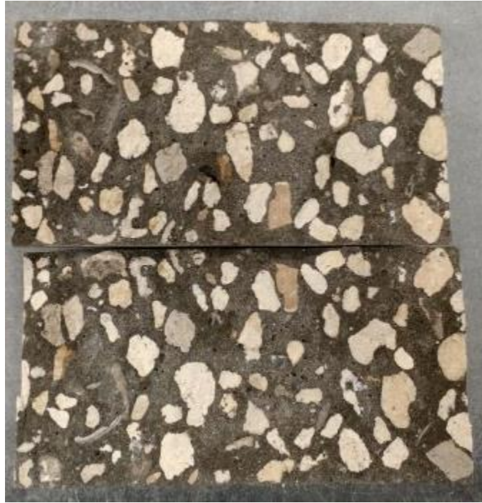
Figure 6-6. Tensile specimen with transgranular fractures.
