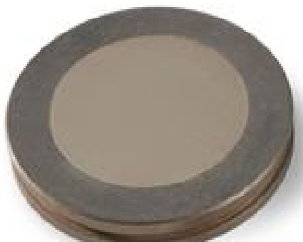
Figure 3-5. X-ray diffraction backfilled sample holder with powder sample.
