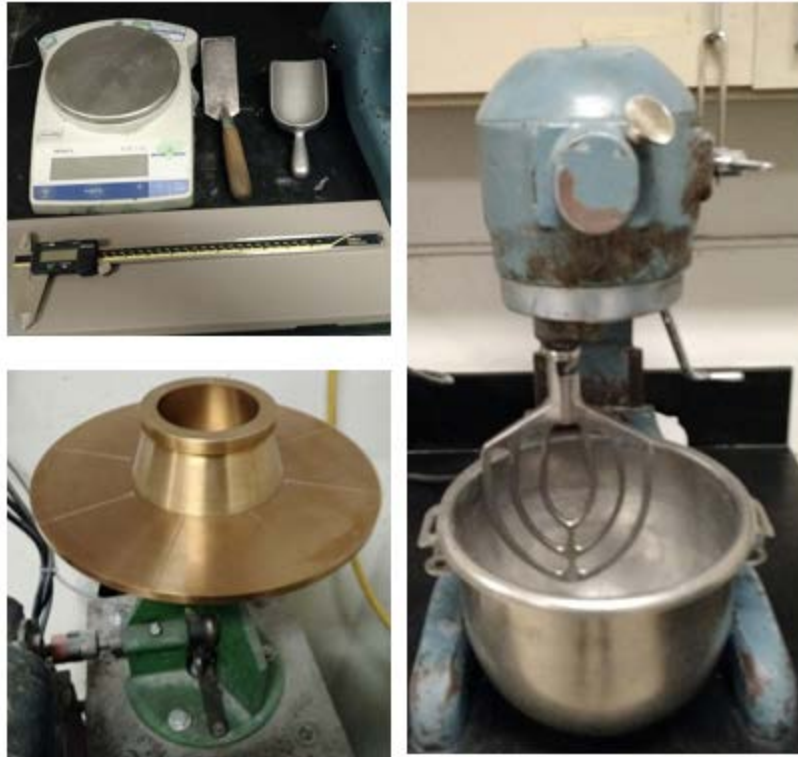
Figure 5-4. Upper left: scale, caliper, trowel and scoop. Bottom Left: flow table with removable brass cone mold. Right: twelve-quart stand mixer with stainless steel paddle and bowl.
