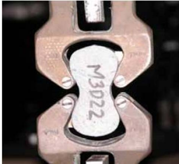
Figure 5-1. Tensile briquette in grips during testing [224].
