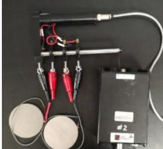
Figure 6-13. CNS Farnell™ surface resistivity probe, with electrical leads connecting the probe to the steel plates.
