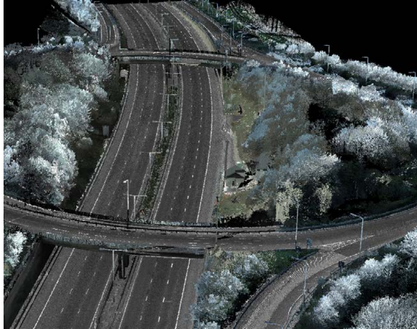
Figure 4 Highway Mobile LiDAR Data
