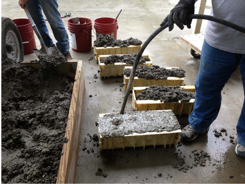
Figure 9. Fabricating Flexural Strength Specimens
