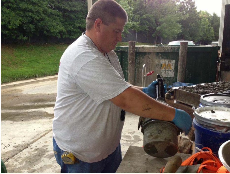
Figure 7. Air Content Testing (Volumetric Method)
