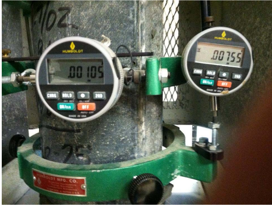
Figure 15. Modulus of Elasticity and Poisson's Ratio Testing
