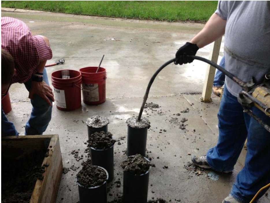
Figure 8. Fabricating Compressive Strength and Modulus of Elasticity Specimens
