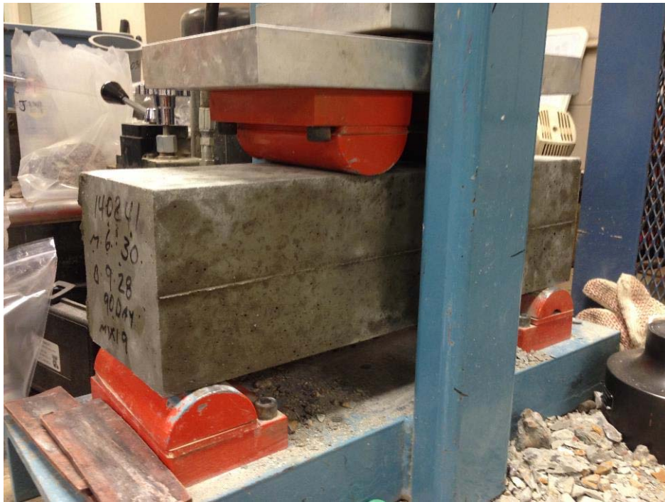
Figure 14. Flexural Strength Testing
