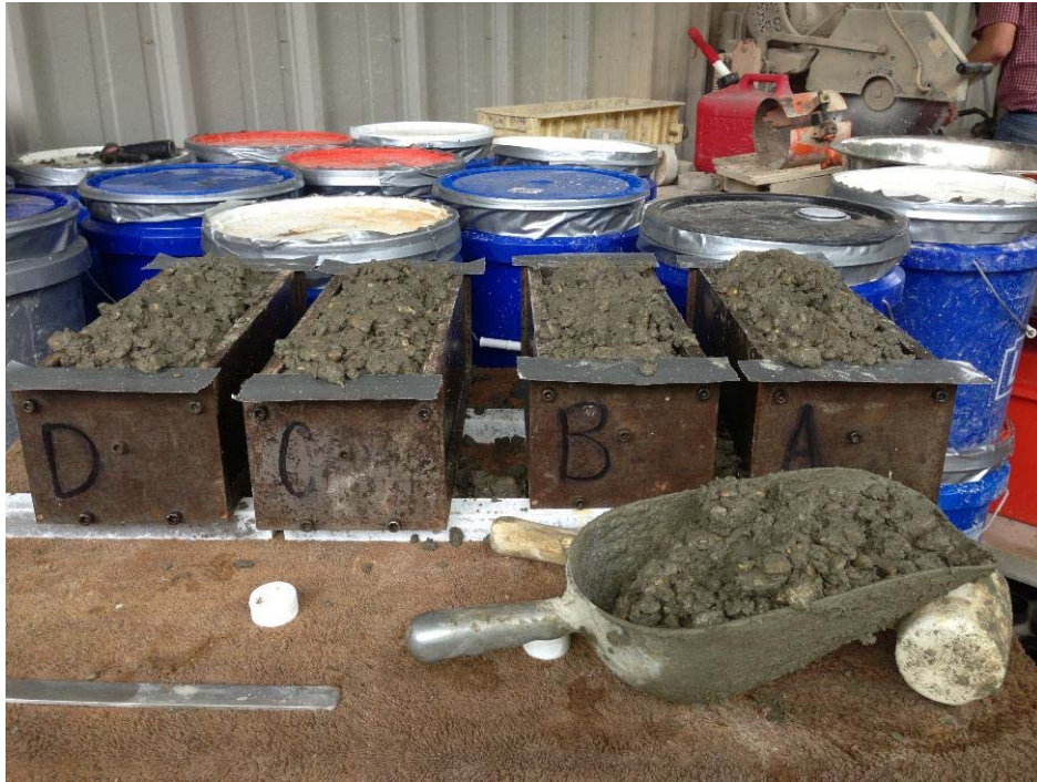
Figure 11. Fabricating Length Change Specimens
