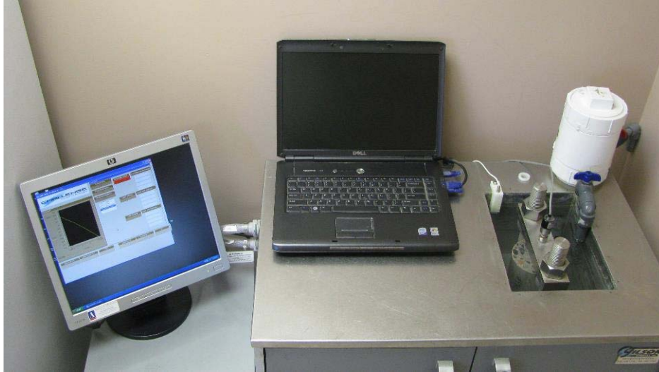
Figure 16. Coefficient of Thermal Expansion Testing (Photograph Courtesy of American Engineering Testing, Inc.)
