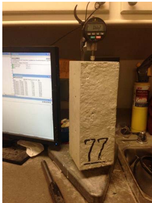
Figure 20. Comparator Reading of Specimen
