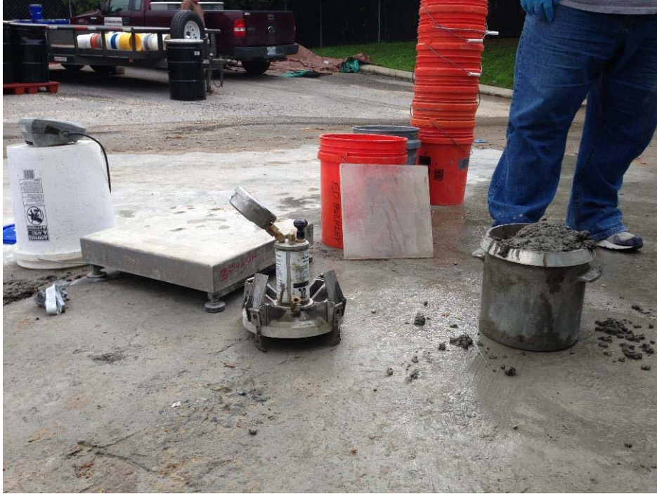
Figure 5. Density and Air Content (Pressure Method) Testing
