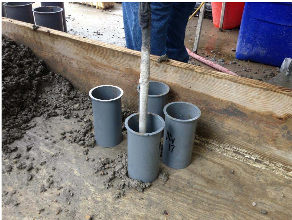
Figure 10. Fabricating Coefficient of Thermal Expansion Specimens
