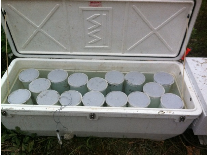
Figure 3-11: Initial Curing of Molded Cylinders
