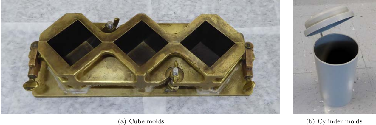
Figure 3.7: Cube and cylinder molds
