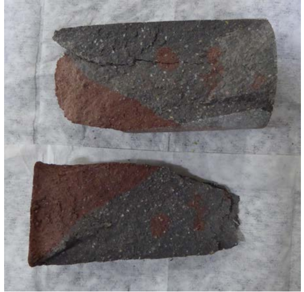
(b) Cylindrical cored from horizontal volume (West face) after compression failure
