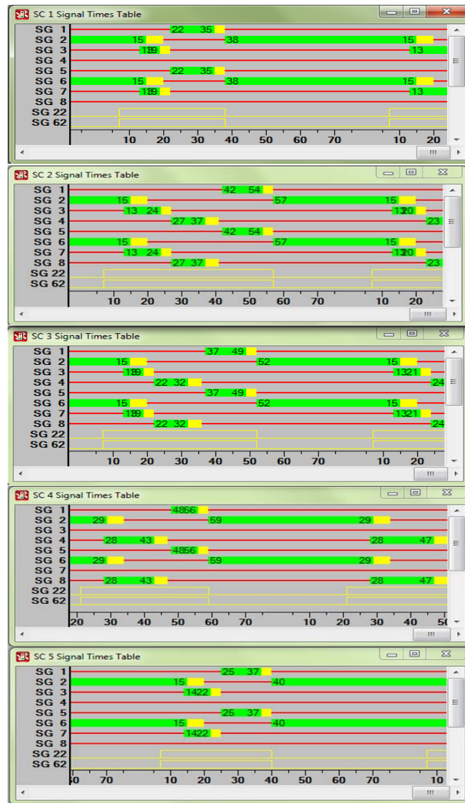
Figure 7.2 Actuated signal timing for the 5 coordinated intersections
