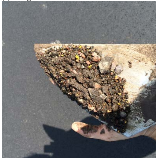
(c) Material that was underneath the core taken directly on the centerline joint
