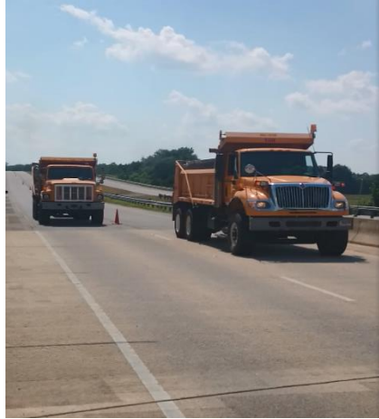
FIGURE 2-17 Two trucks crossing the bridge at the same time
