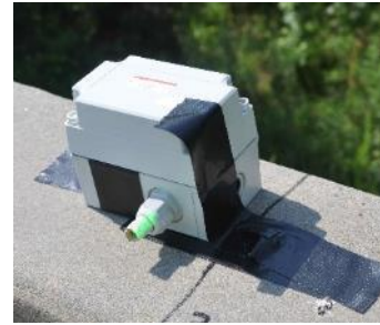
(c) (d) FIGURE 2-3 Truck position sensor: (a) laser emitter; (b) laser receiver; (c) instrumentation plan; (d) laser receiver installed on the bridge
