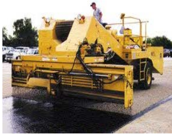
Figure A-56: Chip Spreader
