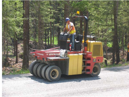
Figure A-57: Pneumatic Tire Roller
