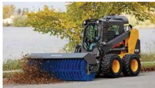
Figure A-60: Brooming Existing Surface
