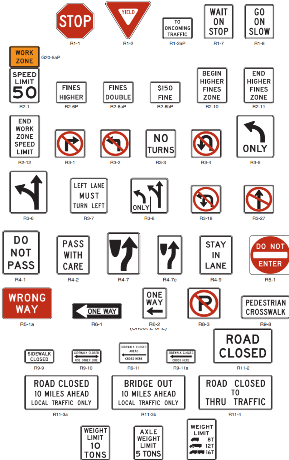
Figure A-42: Regulatory Signs and Plaques in Temporary Traffic Control Zones
