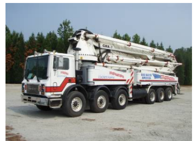
Figure A-61: Pump Truck
