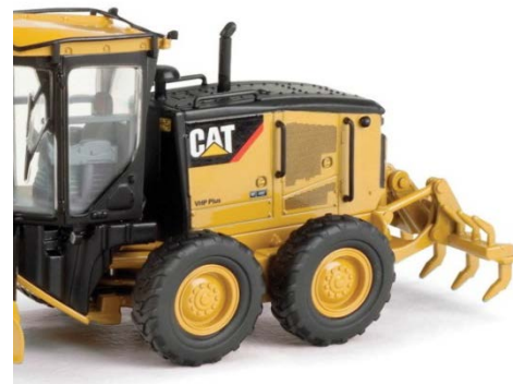
Figure A-34: Grubbing Fork Attached to Motor Grader
