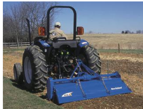
Figure A-33: Tractor with Tiller Attachment
