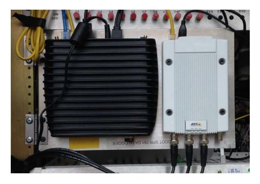
Figure 4.3: FitPC and Axis Encoder
