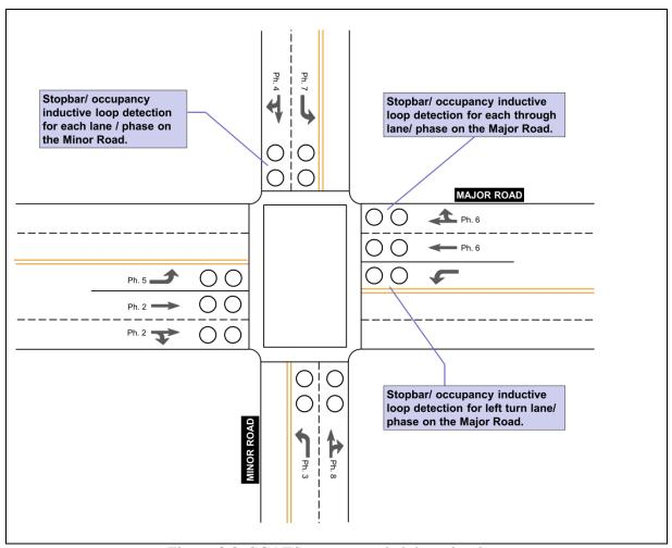
Figure 8.3: SCATS recommended detection layout
