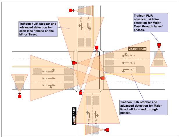
Figure 8.12: Traficon FLIR thermal detector layout for stop bar and advanced detection for Major Road and Minor Road approaches
