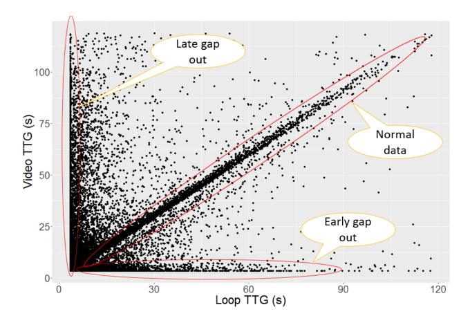
Figure 6.10: Loop TTGs vs Video TTGs of All the Coupled Advance Sensors
