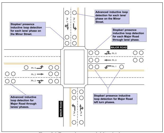
Figure 8.6: Transcend recommended detection layout
