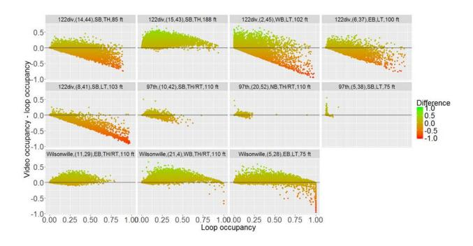
Figure 6.1: Loop Occupancy vs Occupancy Difference of Loop Sensors and Video Sensors
