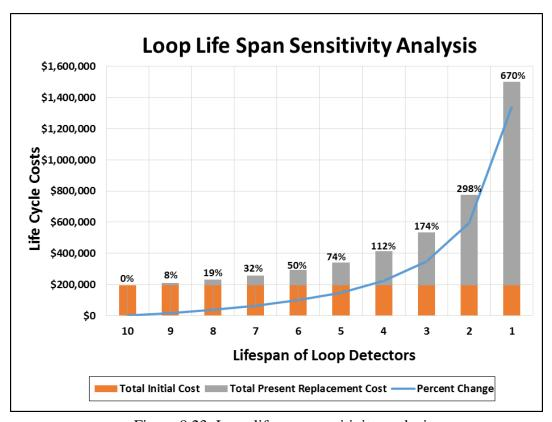
Figure 8.23: Loop life span sensitivity analysis
