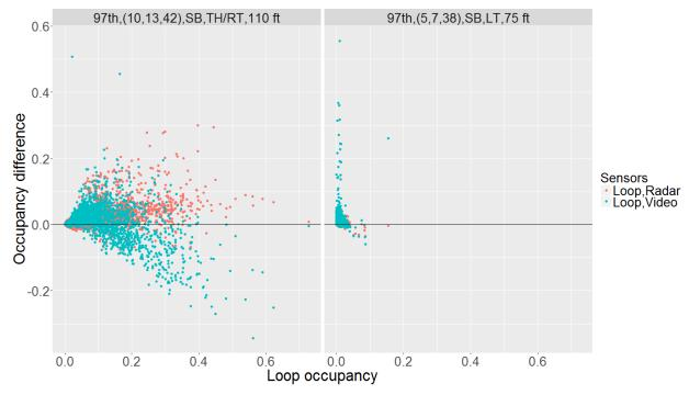
Figure 6.15 Occupancy Difference of Radar and Loop Sensors and Occupancy Difference of Video and Loop Sensors
