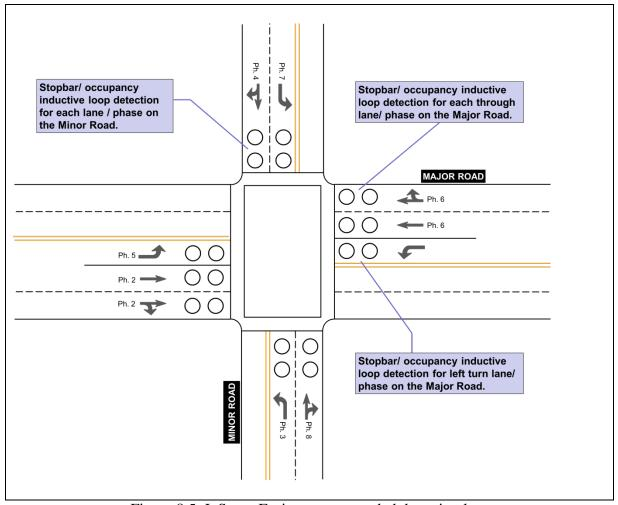
Figure 8.5: InSync: Fusion recommended detection layout
