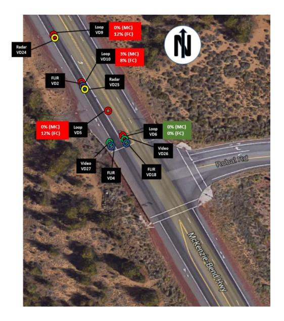
Figure 5.4: Graphic representation of ground truth results at US 20 & Robal Road
