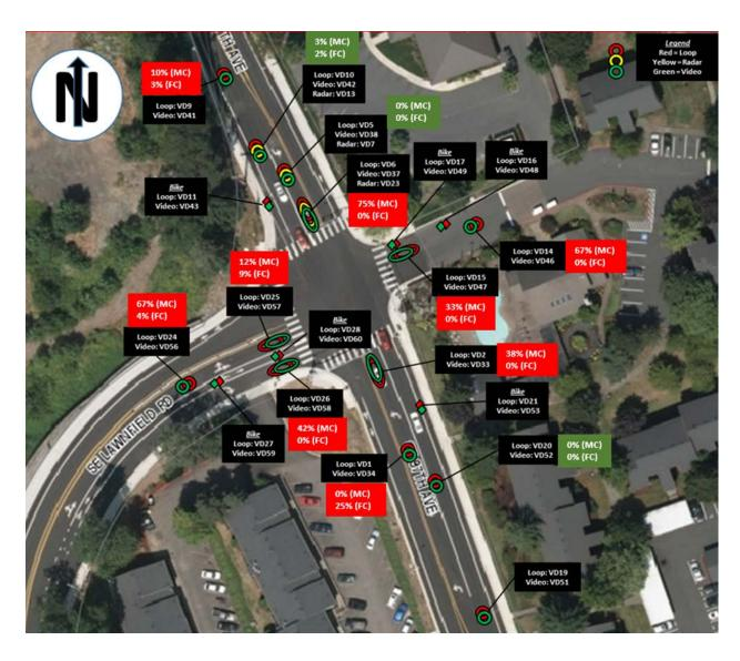
Figure 5.3: Graphic Representation of Ground Truth Results at 97th Avenue & SE Lawnfield Road
