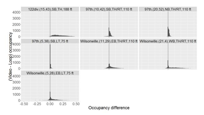
Figure 6.8: Histogram of the Occupancy Differences of Coupled Loop and Video Advance Sensors
