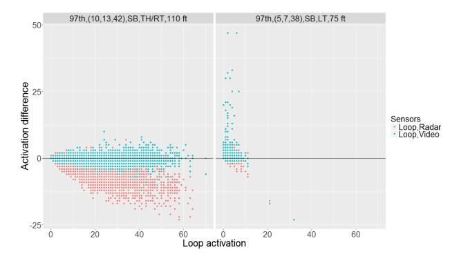
Figure 6.13: Activation Difference of Radar and Loop Sensors and Activation Difference of Video and Loop sensors
