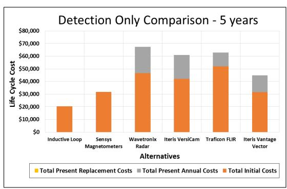
Figure 8.18: Detection only comparisons for 1 intersection over 5 years
