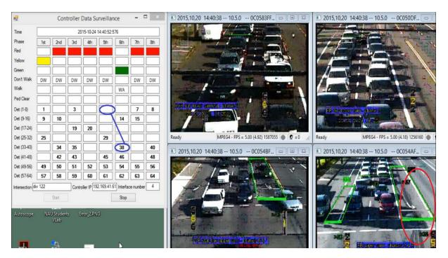
Figure 7.7: Video Sensor 38 Was Stuck in "ON" Status When No Vehicles Existed
