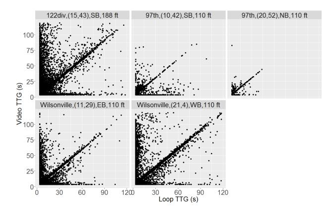
Figure 6.12: Loop TTGs and Video TTGs of Each Pair of Advance Sensors
