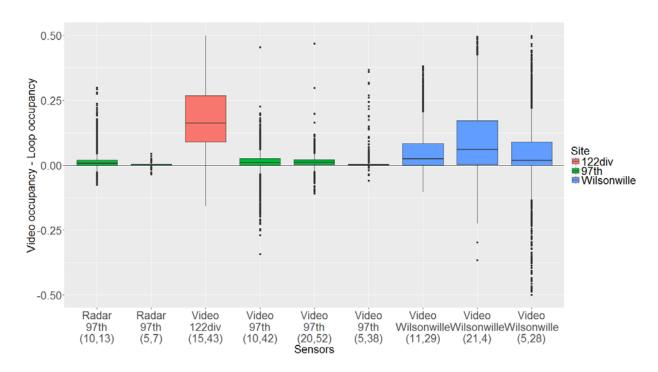
Figure 6.20: Occupancy Differences of Advance Sensors
