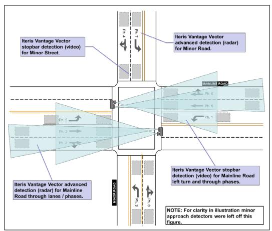
Figure 8.13: Iteris Vantage Vector hybrid detector layout for stop bar and advanced detection for Major Road and Minor Road approaches
