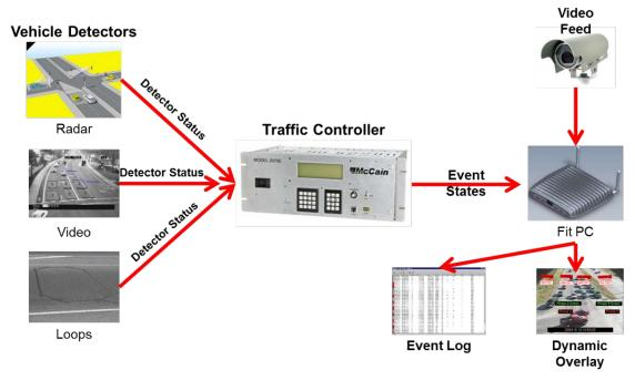
Figure 4.1: Data Structure of Logging Module
