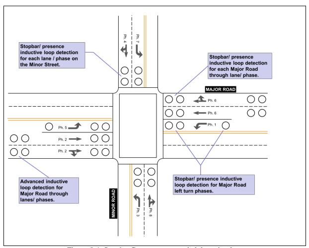
Figure 8.4: SynchroGreen recommended detection layout
