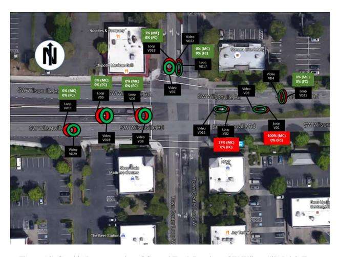
Figure 5.2: Graphic Representation of Ground Truth Results at SW Wilsonville Rd & Town Center Loop West
