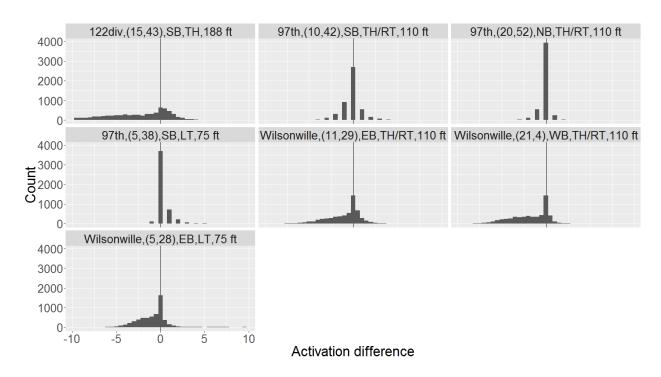
Figure 6.5: Histograms of Activation Differences of Coupled Loop and Video Advance Sensors
