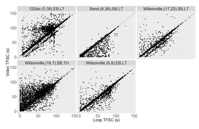
Figure 7.6: Loop TFSCs vs Video TFSCs of Each Pair of Stop bar Sensors
