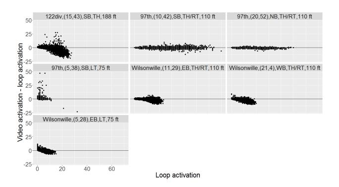
Figure 6.4: Activation Differences of Coupled Loop and Video Advance Sensors
