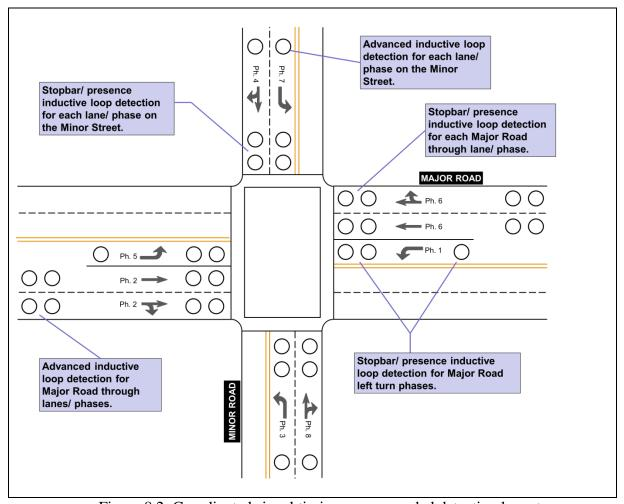
Figure 8.2: Coordinated signal timing recommended detection layout
