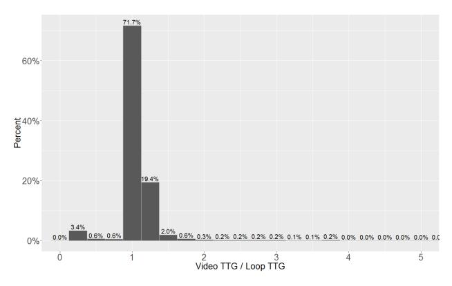
Figure 7.2: Histogram of the Ratio of Video TTGs to Loop TTGs
