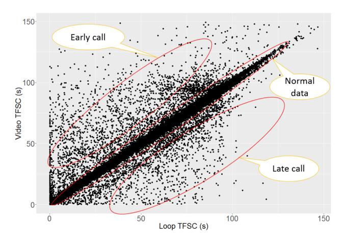
Figure 7.4: Loop TFSC vs Video TFSC of Stop bar Sensors
