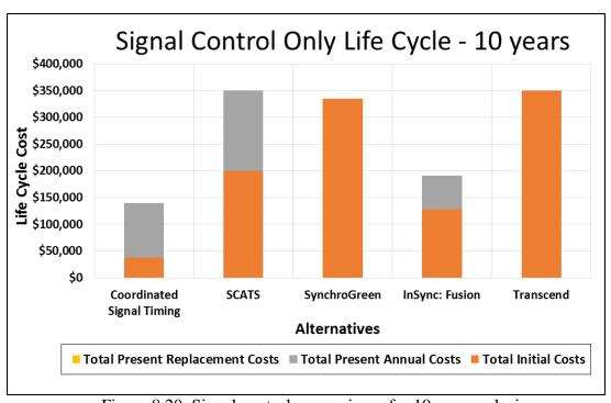
Figure 8.20: Signal control comparisons for 10 year analysis
