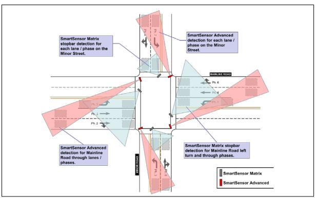
Figure 8.10: Wavetronix radar detection layouts for both stop bar and advanced detection for Major Road and Minor Road approaches
