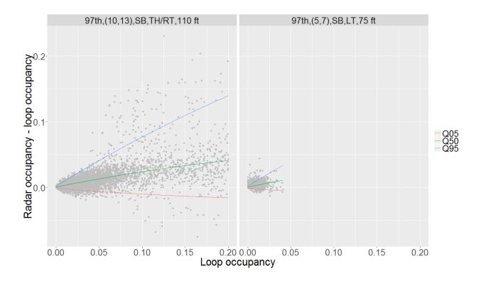
Figure 6.16: Fitted Occupancy Differences with the Quantile Regression Model of Advance Radar Sensors
