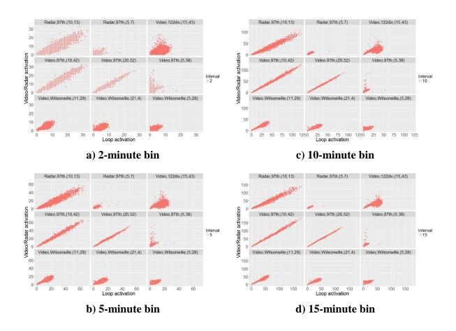
Figure 6.2: Loop activation vs video/radar activation aggregated by 2min, 5min, 10min, and 15min
