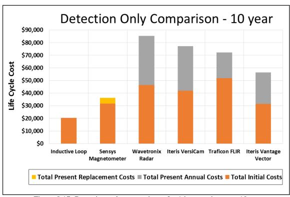
Figure 8.17: Detection only comparisons for 1 intersection over 10 years
