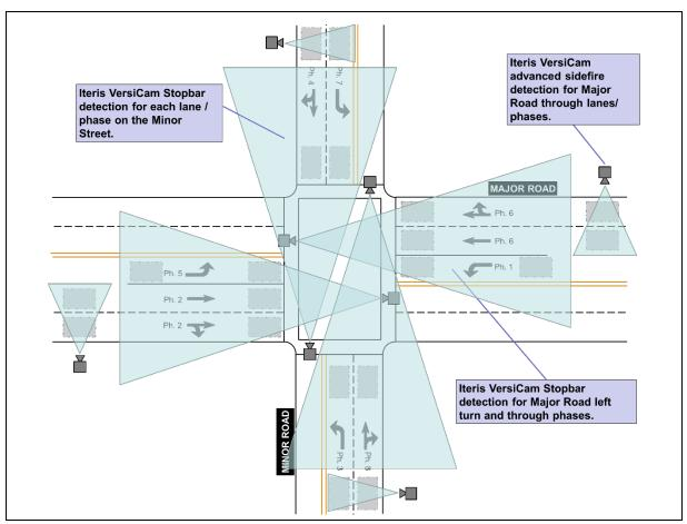
Figure 8.11: Iteris VersiCam video detector layouts for stop bar detection for Major Road and Minor Road approaches
