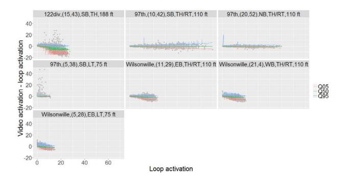
Figure 6.6: Estimated Quantile vs Field Observations of Activation Difference of Advance Video Sensors
