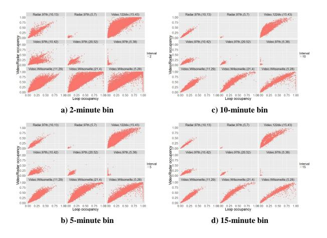
Figure 6.3: Loop occupancy vs video/radar occupancy aggregated by 2min, 5min, 10min, and 15min
