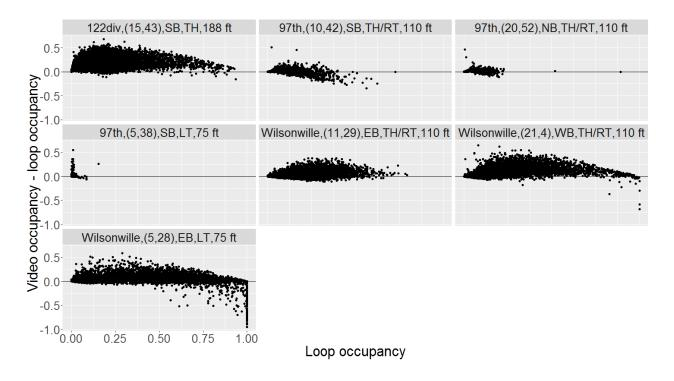
Figure 6.7: Occupancy Difference of Coupled Loop and Video Advance Sensors
