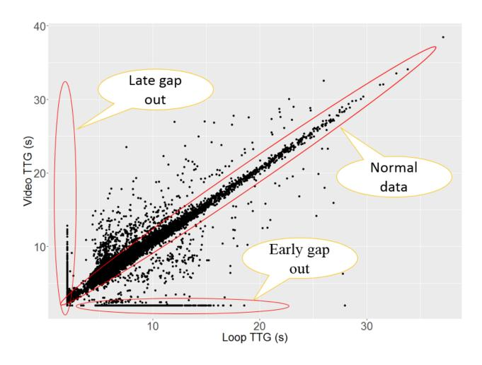
Figure 7.1: Lg1Vg1 TTG Data of Coupled Stop bar Sensors
