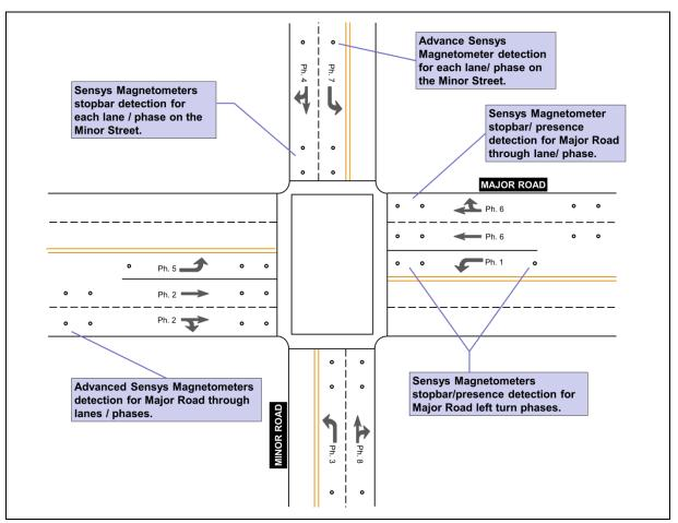
Figure 8.9: Sensys Magnetometers detection layouts for both stop bar and advanced detection for Major Road and Minor Road approaches
