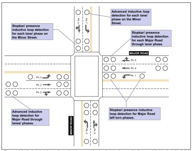
Figure 8.8: Inductive loop detection layouts for both stop bar and advanced detection for Major Road and Minor Road approaches
