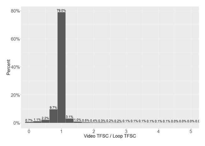
Figure 7.5: Histogram of the Ratio of Video TFSC to Loop TFSC
