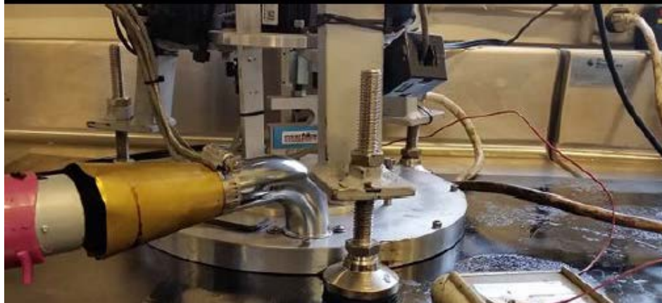
Figure 7.6: A new temperature control system for OFTCT to reduce measurement variability
