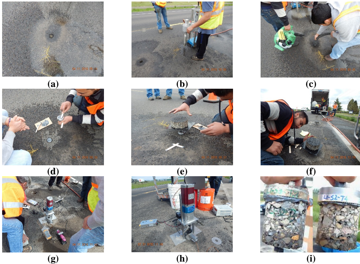
Figure 6.3: General procedure followed for OFTT field experiments
