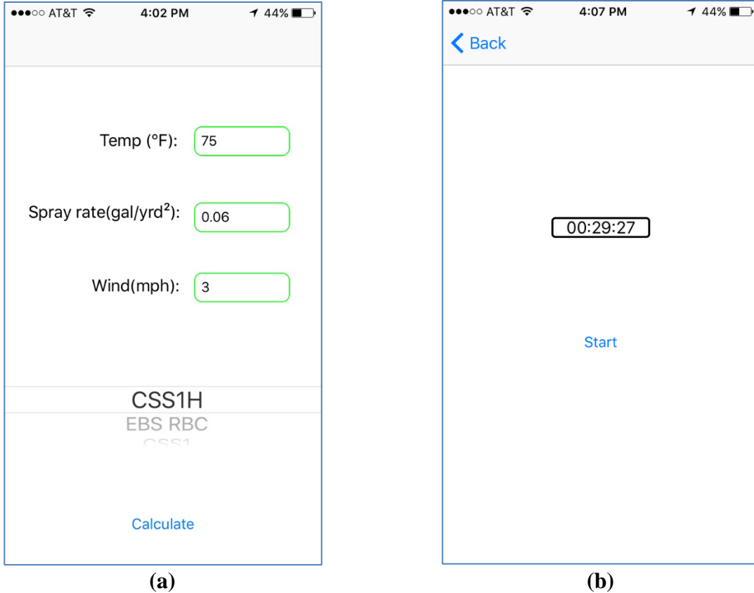
Figure 4.7: Screenshot taken from smartphone app (IOS) developed for tack coat curing time (a) user input (b) countdown timer
