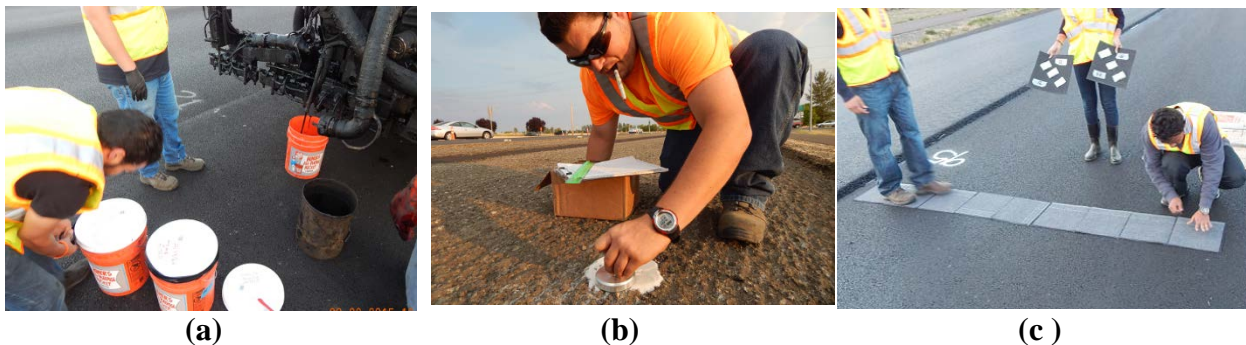
Figure 3.1: Experiments conducted to evaluate tack coat application methods and procedures (a) emulsion sampling for laboratory tests (b) sand patch texture measurements (c) application rate measurement
