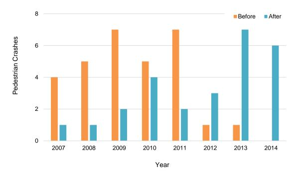
Figure 4.4: Pedestrian Crashes Before and After a Pedestrian Crossing Enhancement Installation
