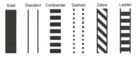
Figure 2.1: Common Crosswalk Markings (Zegeer et al. 2001)
