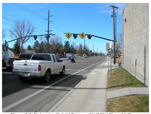
Figure 2.5: Pedestrian Hybrid Beacon (HAWK), Photo N. Foster
