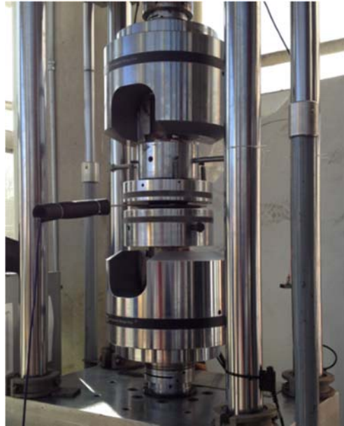
Figure B-1. MTS hydraulic press applying load to Geokon Pressure Cell
