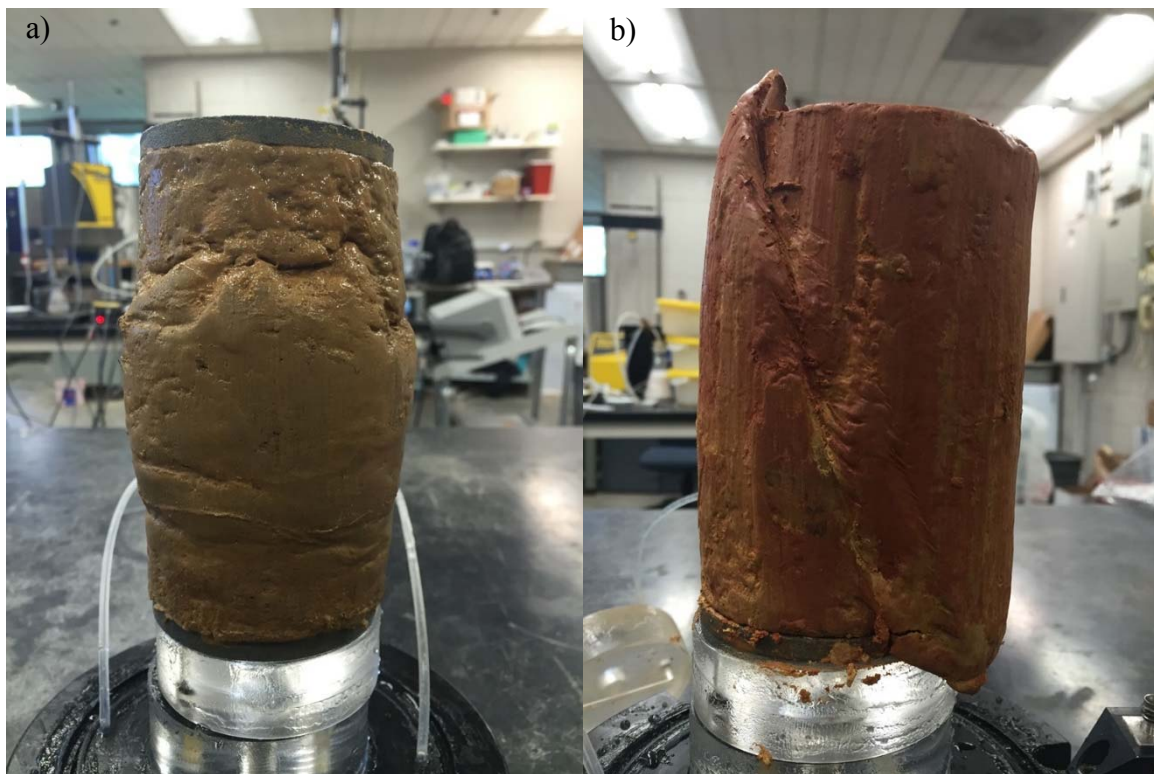
Figure 4-7. CU triaxial specimens at failure state a) A-4 soil & b) A-7-5 soil.
