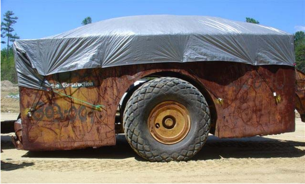
Figure 8-24. Proof roll trailer (courtesy M. Valiquette, NCDOT, Borden et al., 2010)
