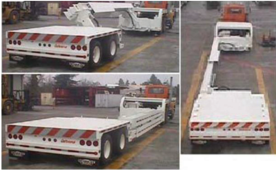
Figure 3.37 Balsi Beam mobile barrier system (California Department of Transportation, 2010).
