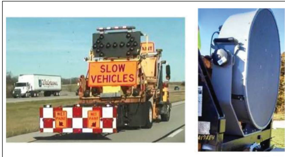
Figure 3.16 Construction vehicle with TMA for DAS (Brown et al., 2015).
