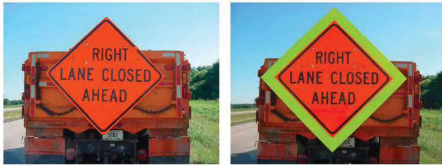
Figure 3.35 Evaluation of fluorescent-yellow-green (FYG) background against orange colored TMA signs (Kamyab & Storm, 2001).
