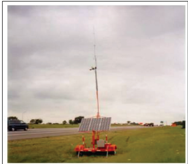
Figure 3.18 Sensor station trailer configured with traffic sensor, microwave antenna and solar panel (Zwahlen, 2002).
