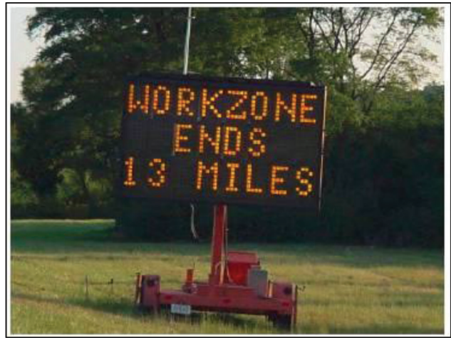
Figure 3.17 Changeable message sign in TIPS system displaying distance to the end of the work zone (Zwahlen, 2002).
