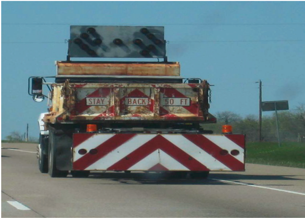
Figure 3.34 Example of a TMA in use during a mobile operation (Ullman et al., 2011).
