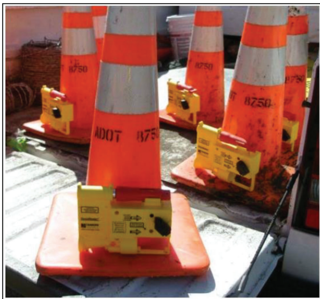
Figure 3.15 SonoBlaster!® Work Zone Intrusion Alarm (Krupa, 2010).
