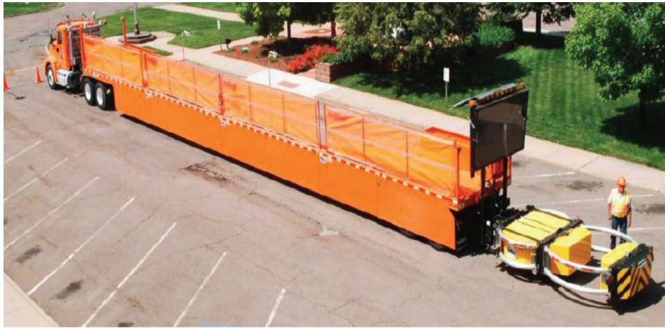
Figure 3.38 Mobile barrier trailer-1 (MBT-1) (Mobile Barriers LLC, 2009).
