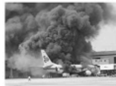
Fire on Thai Airways Boeing 707-400 on 3rd March 2001, Bangkok, Thailand after centre fuel tank explosion. Picture source: NTSB memory.
