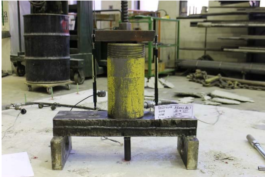
Figure B.37 Complete assembly and specimen prior to testing for P60-AE-3
