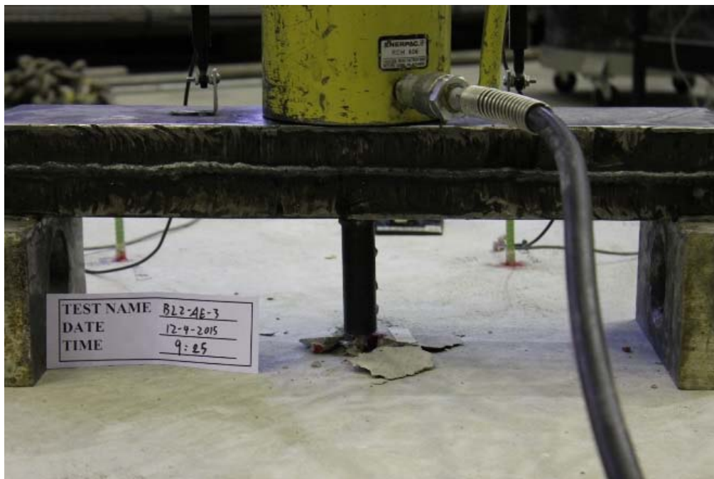
Figure B.8 Detailed view of the reinforcement at failure for BL-AE-3
