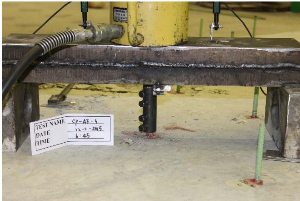
Figure B.26 Detailed view of the reinforcement at failure for CP-AE-3
