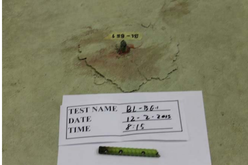
Figure 4.18 Representative failure mode for BL-BE of combined failure (concrete breakout and steel rupture)
