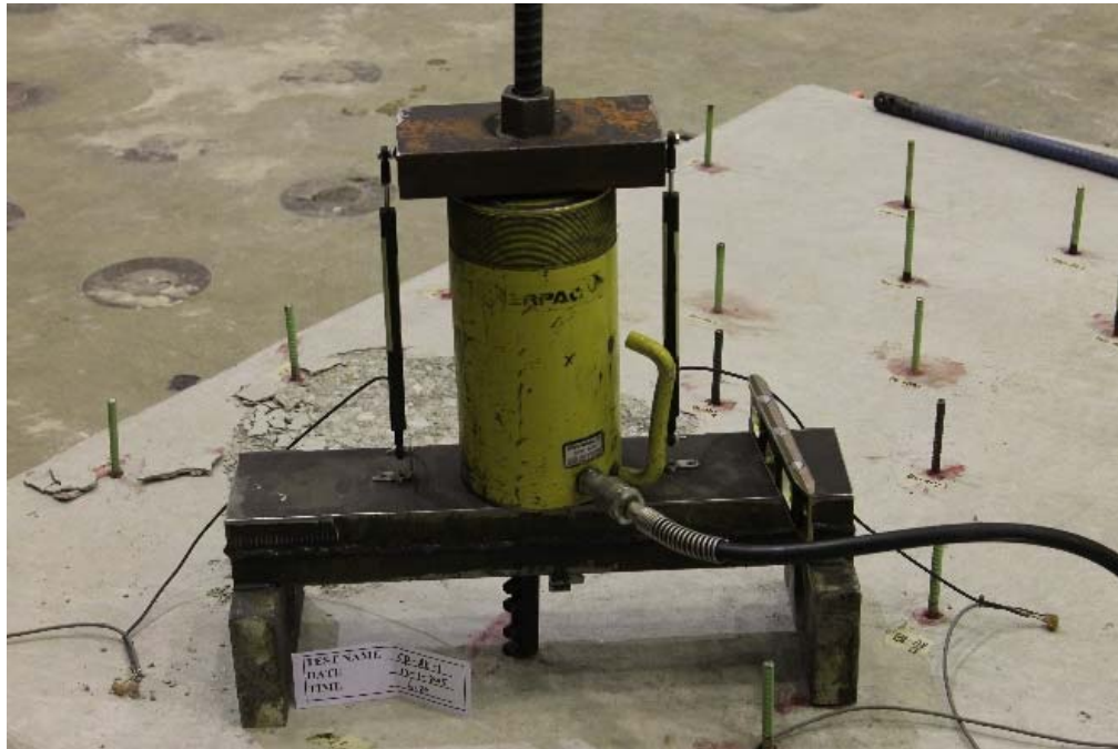
Figure B.19 Complete assembly and specimen prior to testing for CP-AE-1
