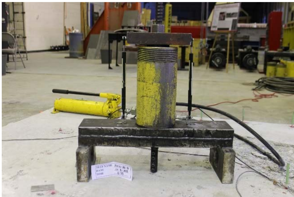
Figure B.39 Complete assembly and specimen prior to testing for P60-AE-4
