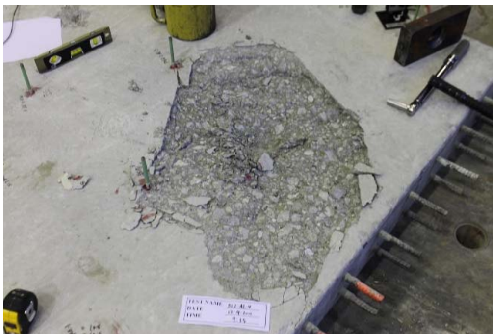
Figure B.12 Specimen details after testing for BL-AE-4
