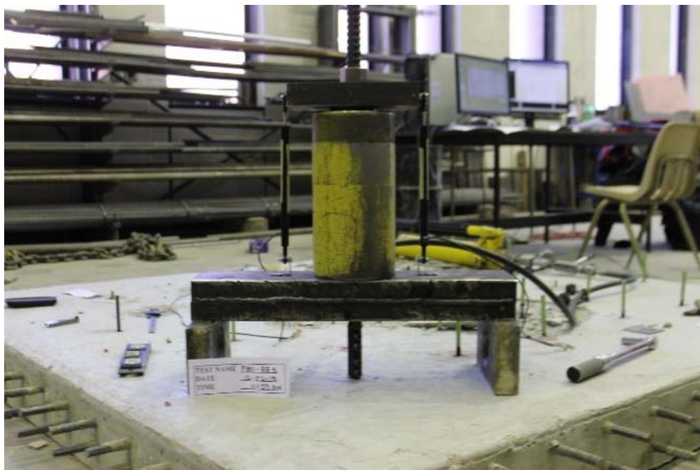
Figure B.46 Complete assembly and specimen prior to testing for P80-AE-5
