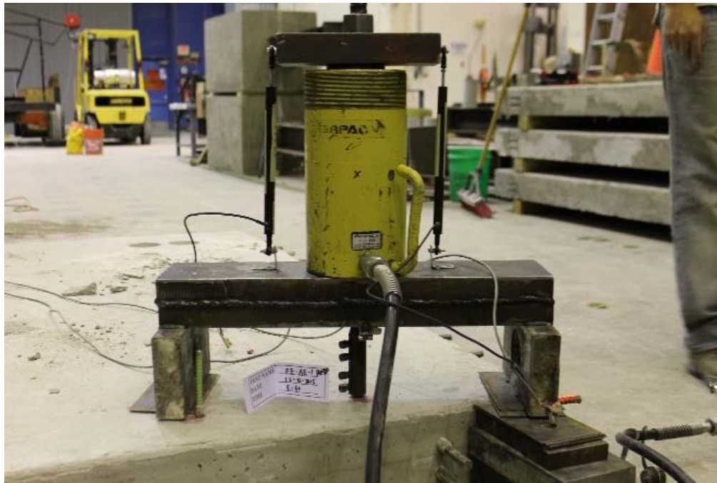
Figure B.55 Complete assembly and specimen prior to testing for EE-AE-1
