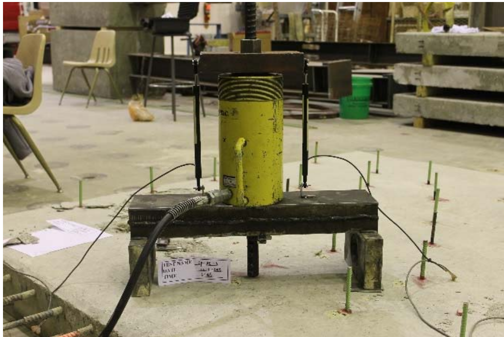
Figure B.25 Complete assembly and specimen prior to testing for CP-AE-3
