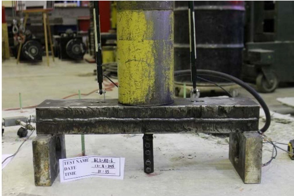
Figure B.13 Complete assembly and specimen prior to testing for BL-AE-5
