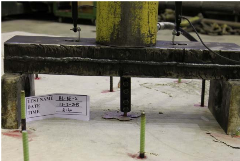
Figure B.53 Detailed view of the reinforcement at failure for BL-BE-2
