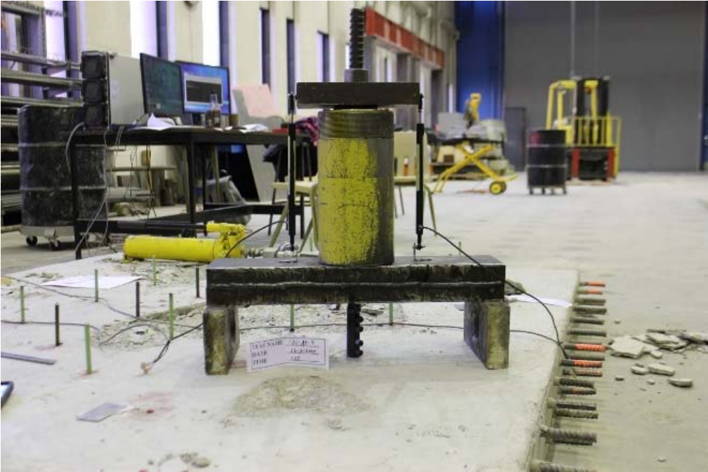
Figure B.44 Complete assembly and specimen prior to testing for P80-AE-4
