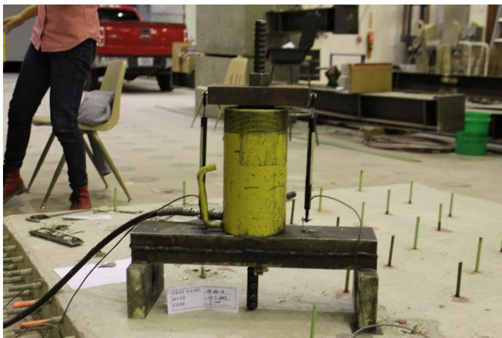
Figure B.28 Complete assembly and specimen prior to testing for CP-AE-4
