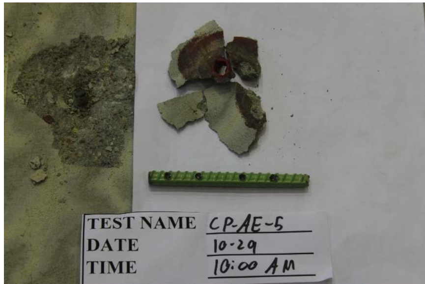
Figure 4.3 Representative failure mode for CP-AE in 5.8 ksi compressive strength concrete
