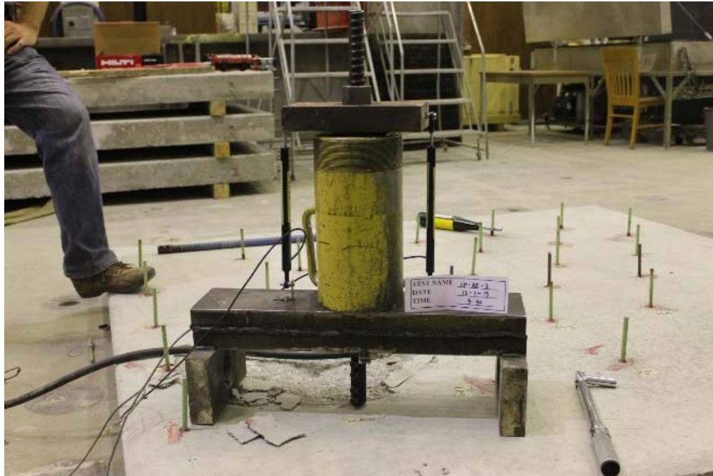
Figure B.22 Complete assembly and specimen prior to testing for CP-AE-2
