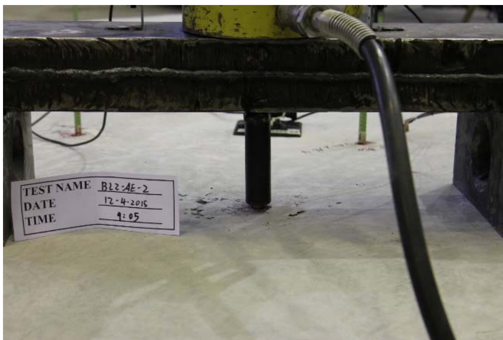
Figure B.5 Detailed view of the reinforcement at failure for BL-AE-2
