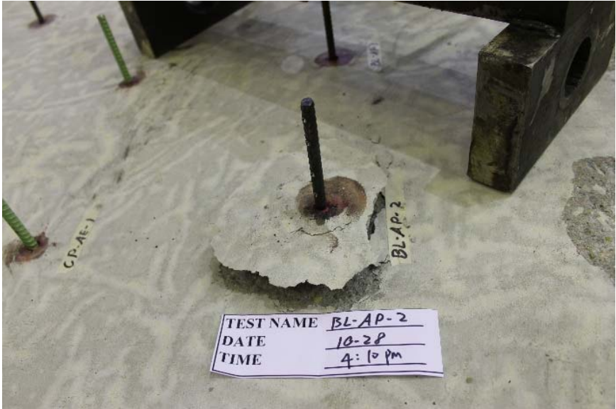
Figure 4.2 Representative failure mode for BL-AP of combined failure in 5.8 ksi compressive strength concrete
