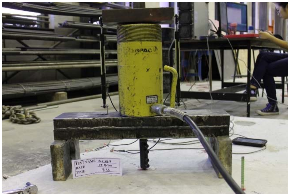
Figure B.10 Complete assembly and specimen prior to testing for BL-AE-4
