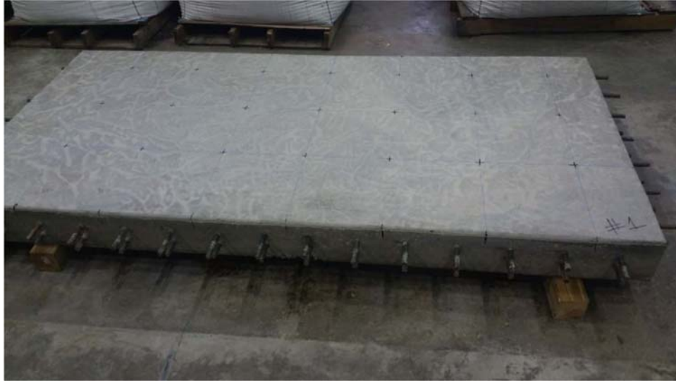
Figure 3.3 The final concrete slab (1-1) with identified locations for test specimens
