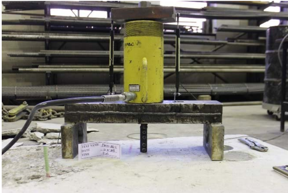
Figure B.33 Complete assembly and specimen prior to testing for P60-AE-1
