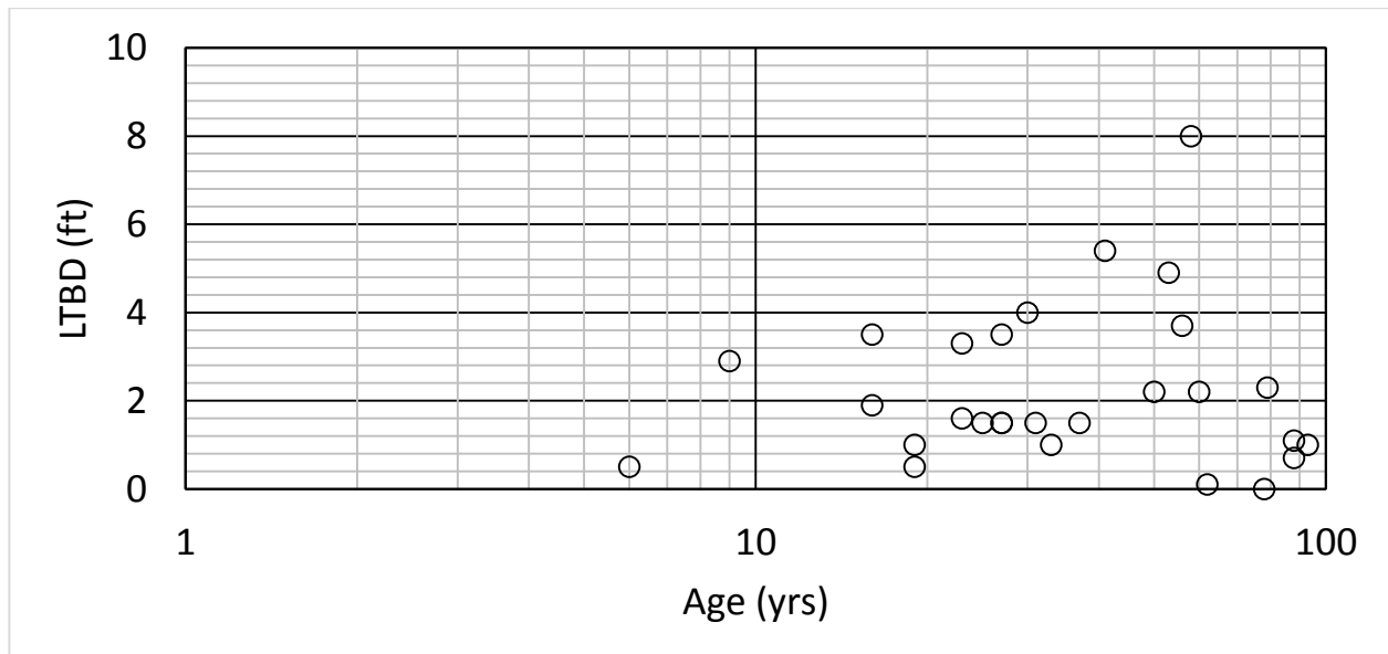
Figure 4.6. Variation of LTBD with structure’s age. Plotted data points for two structures overlapped: the structures have an age of 27 years and an LTBD of 1.5 feet.
