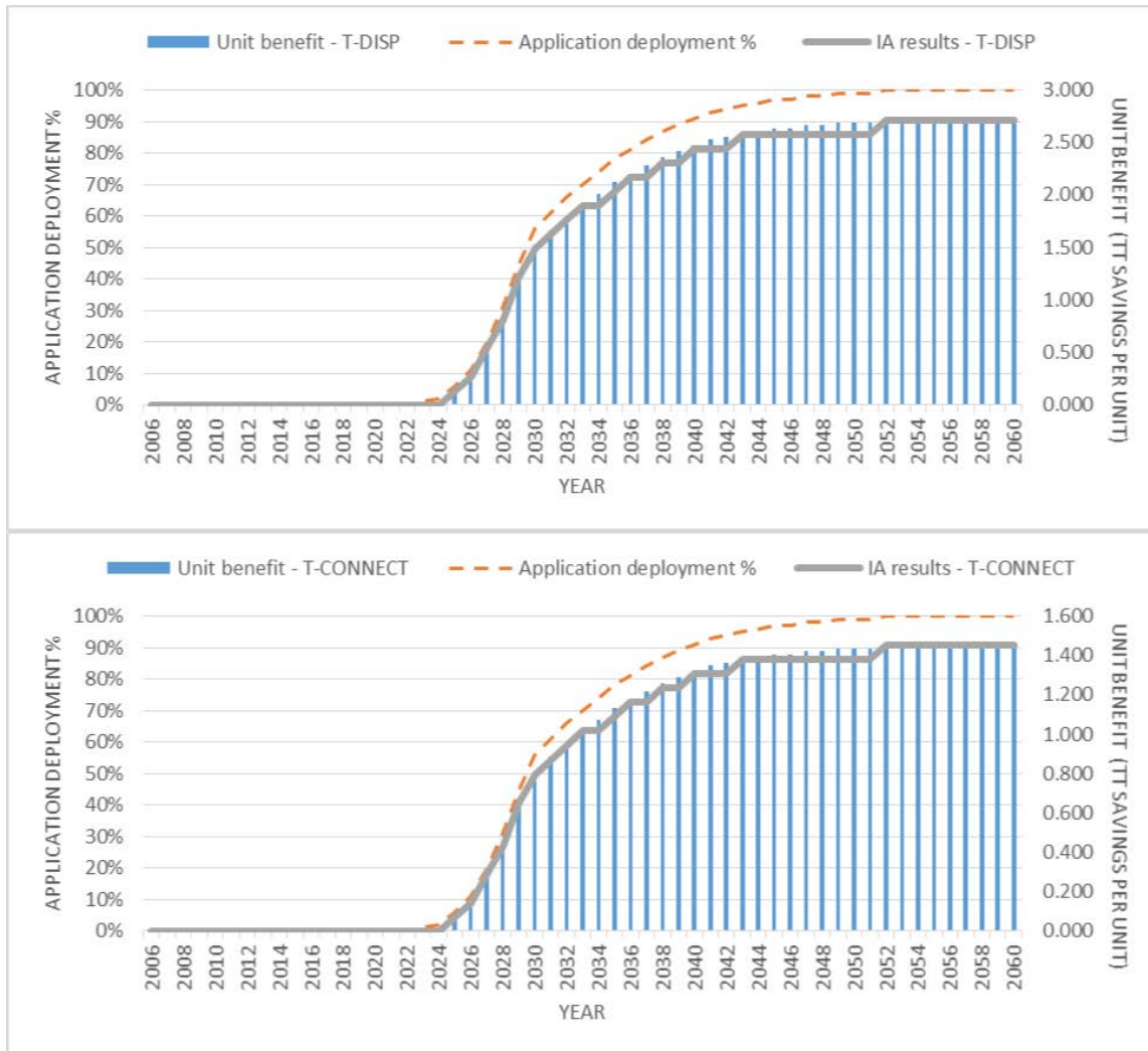
Figure 29. T-DISP and T-CONNECT Mobility Impacts Matched with the Years When the Corresponding CV Penetration Rates are Expected to be Achieved
