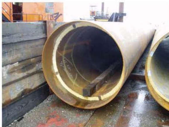
Figure 4. (Left) Sound attenuation methods. The pipe on the left in the picture is a double walled steel pipe with foam layer between walls. The pipe beside it on the right shows a single steel sleeve pipe with a foam layer. (Right) The diagram on the rights shows the effects of sound mitigation methods on the received 90% RMS SPL at four distances from the pile driver: 10 m, 50 m, 100 m, and 1100 m. All piles were 36-inch diameter steel pipes.
