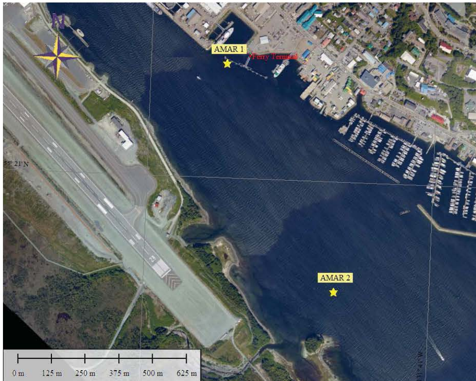
Figure 6. AMAR deployment locations during hydroacoustic monitoring at Ketchikan, Alaska. Aerial orthophotos obtained from NOAA Office for Coastal Management (2016b).
