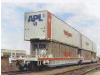
American President Lines' 40-foot "Lo-Pac" demonstration car shows how 40-foot containers can sit atop 40-foot open-tops in a 40-foot well car. The advent of 53-foot boxes complicated this setup, un...
