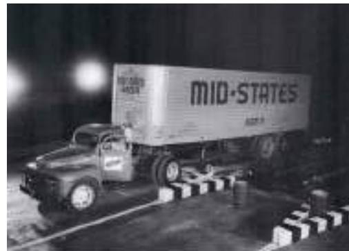
A driver backs his trailer onto the Pennsylvania Railroad's first intermodal flat in March 3, 1955, at PRR's Chicago Yard. It's destined for South-Kearny, N.J. The circus loading process was labor- and time-intensive. (Source: C. Allen, Smithsonian Magazine)
