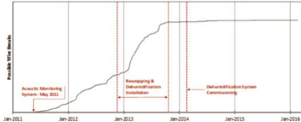
Figure 3-7: Potential wire breaks on the Westbound Bay Bridge [Waldvogel et al, 2016]
