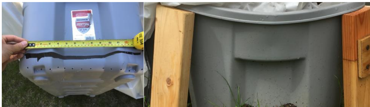
(a) Geotextile opening and drainage holes
