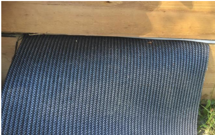
(c) Half-inch opening for testing flume side wall
