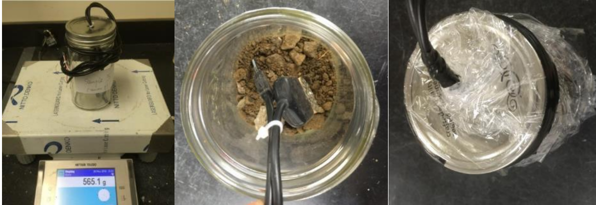
(a) SWCC testing equipment (suction < 1000 kPa)
