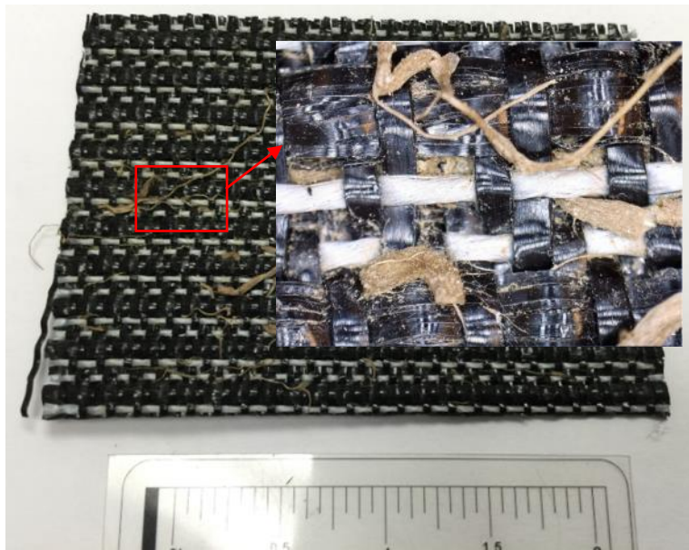
Figure 4.12 Microscopic image of grass-geotextile interaction
