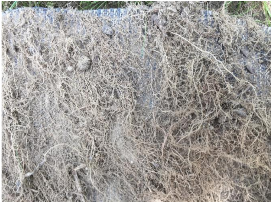
(b) Grass roots penetrating the geotextile
