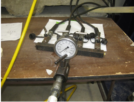
Figure 6.4 Dial Gauge Used for Pressure Readings
