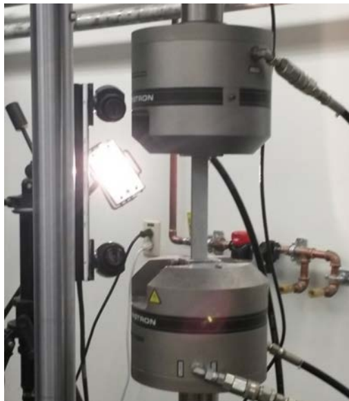
Figure 2.3 Tension Test (ASTM D3039)
