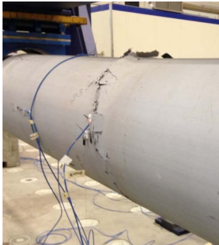
Figure 5.11 Compression Failure of Pile J
