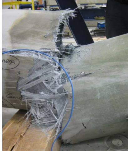
Figure 5.19 Tension Failure of Pile A
