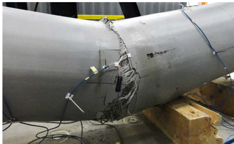
Figure 5.23 Tension Failure of Pile E
