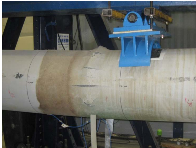
Figure 5.12 Compression Failure of Pile B
