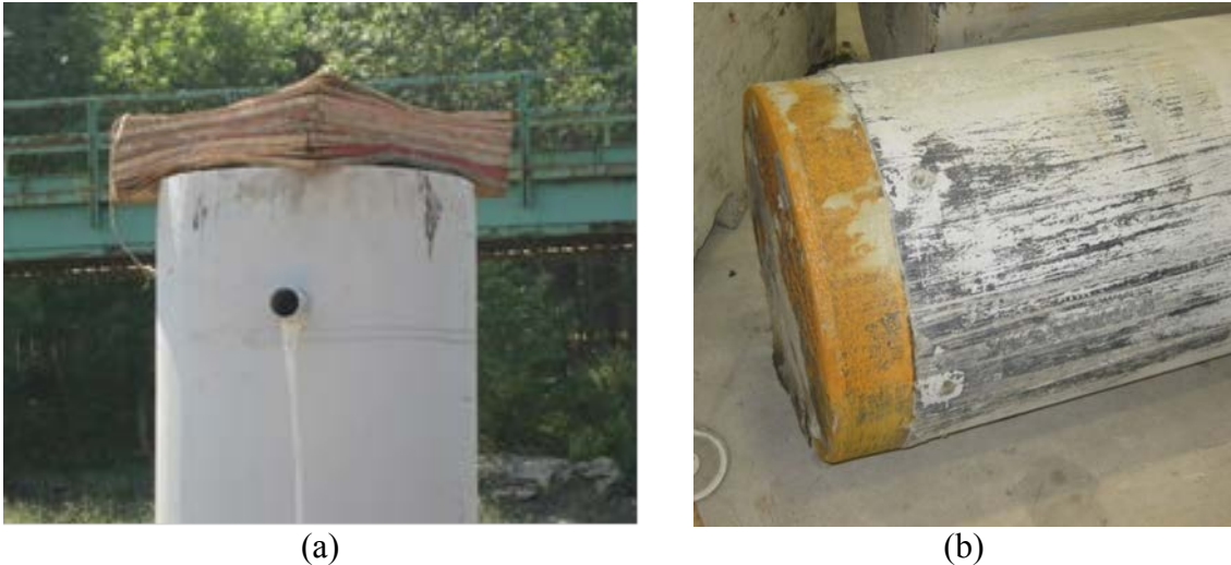
Figure 4.10 Head (a) and Toe (b) of Pile A after Initial Driving
