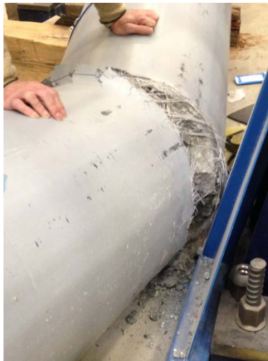
Figure 5.24 Tension Failure of Pile F
