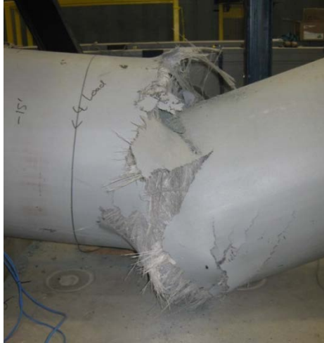
Figure 5.17 Tension Failure of Pile G
