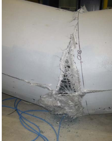
Figure 5.18 Tension Failure of Pile H
