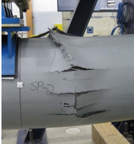
Figure 5.10 Compression Failure of Pile I
