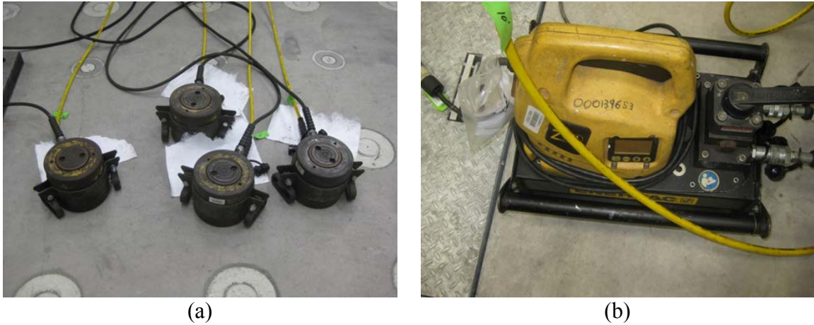
Figure 6.2 150 Ton Enerpac Cylinders (a) and Hydraulic Pump (b)
