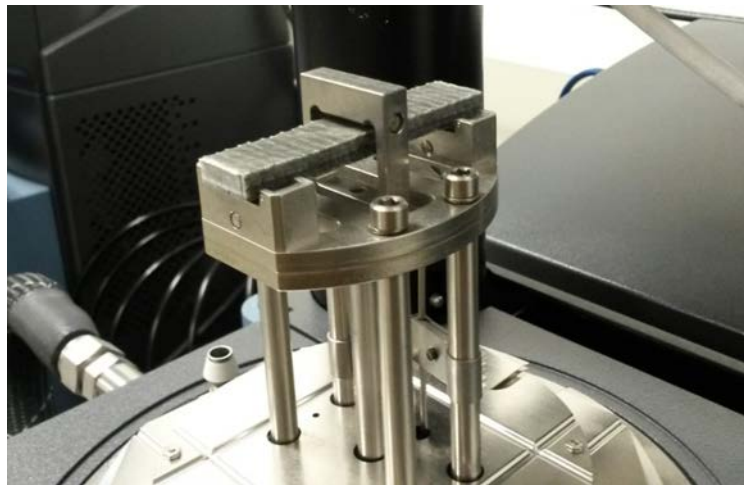
Figure 2.13 Glass Transition Temperature Test (ASTM E1640)
