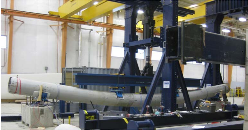
Figure 5.1 Flexural Test Configuration
