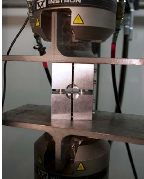
Figure 2.7 Compression Test (ASTM D6641)
