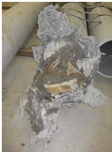
Figure 4.14 Toe of Pile C after Restrike
