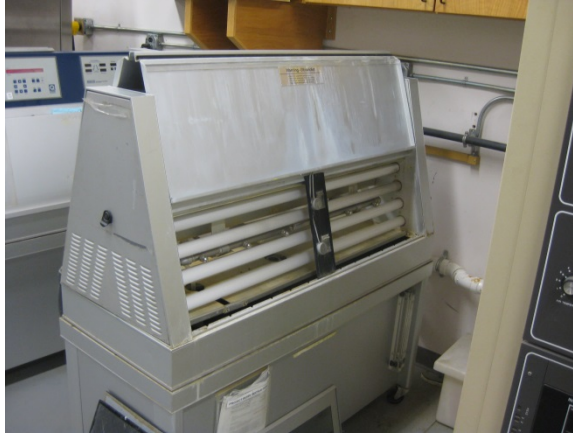
Figure 4 UV/Condensation Humidity Test Chamber
