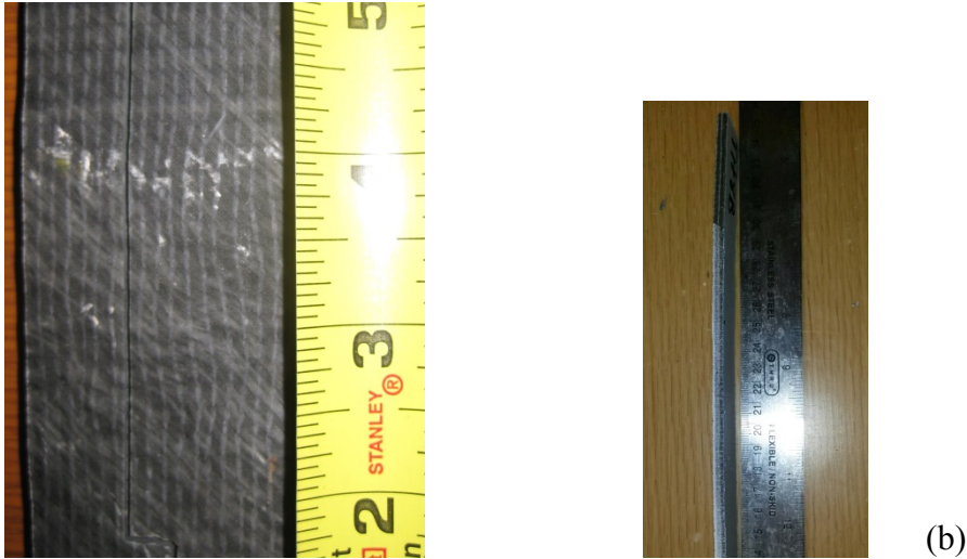
Figure 6 Misaligned Fibers (a) and Warping (b) in Durability Samples
