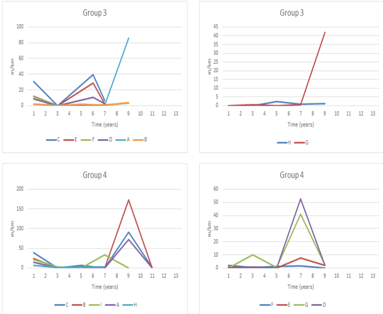
Figure 14. Moderate longitudinal cracking deterioration for Groups 3 and 4
