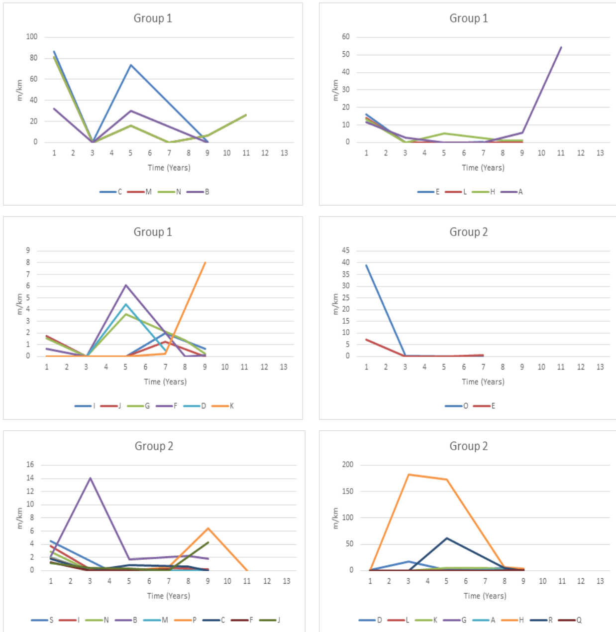
Figure 9. High transverse cracking deterioration for Groups 1 and 2
