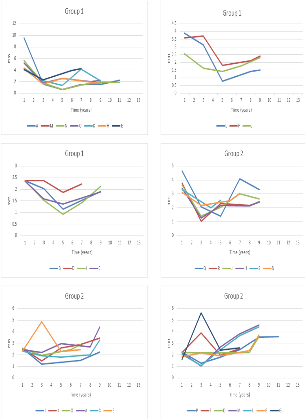
Figure 24. Rut depth for left wheelpath deterioration for Groups 1 and 2
