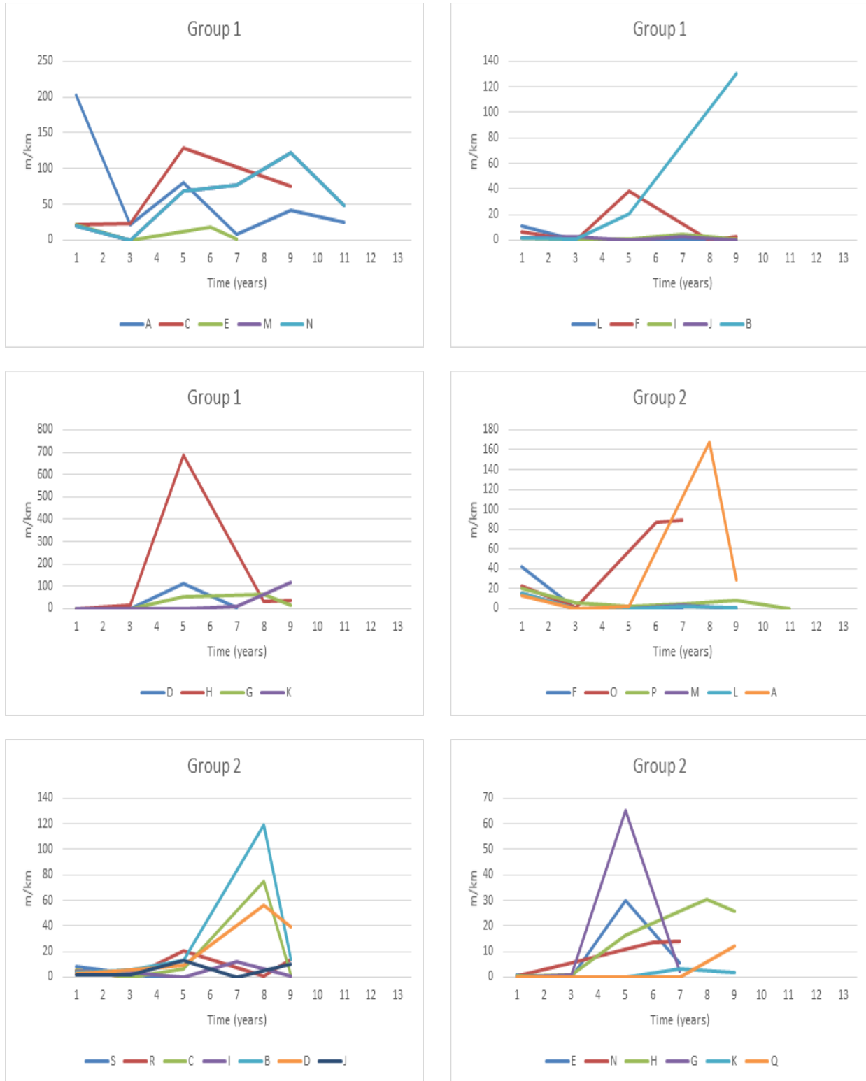
Figure 13. Moderate longitudinal cracking deterioration for Groups 1 and 2
