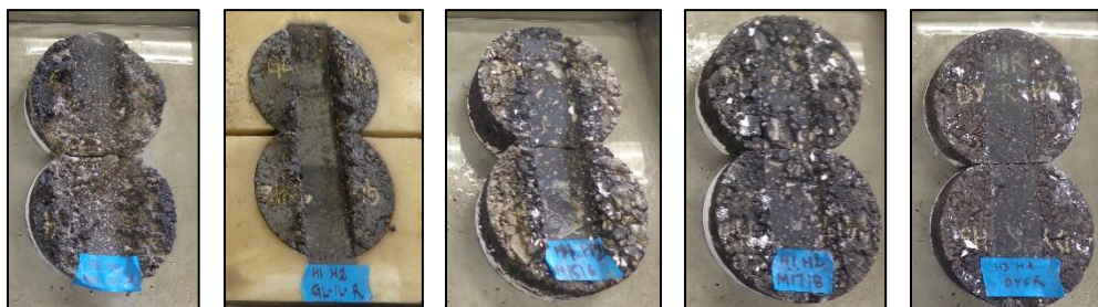
Figure 4-11 From left to right specimens tested by Hamburg: Galesburg Outer Lane, Galesburg Inner Lane, Machesney 15-16, Machesney 17-18, Dyer, respectively
