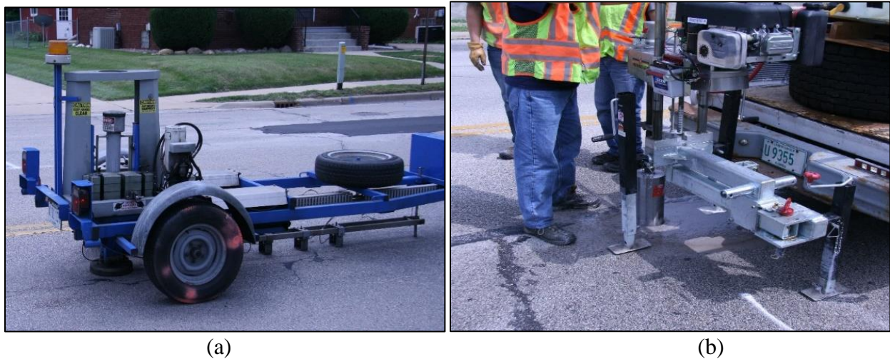
Figure 3-5 (a) FWD measurement before HIR (b) extraction of cores at Galesburg, IL
