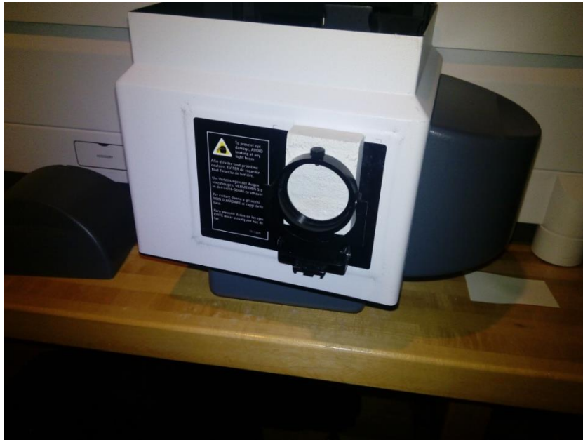
Figure 3-4 Spectrophotometer testing of a photocatalytic mortar sample
