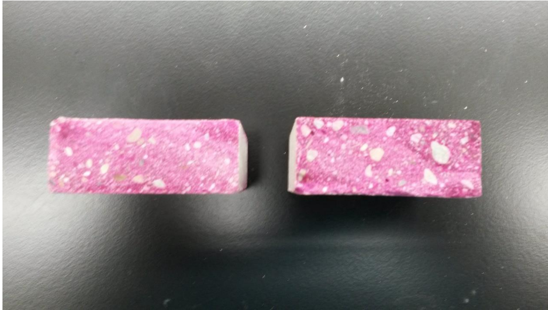
Figure 3-12 Side-by-side image of interior of interior fracture surfaces of non-carbonated (left) and carbonated (right) White TiO 2 , 30% Fly Ash mortar specimens after treatment with phenolphthalein
