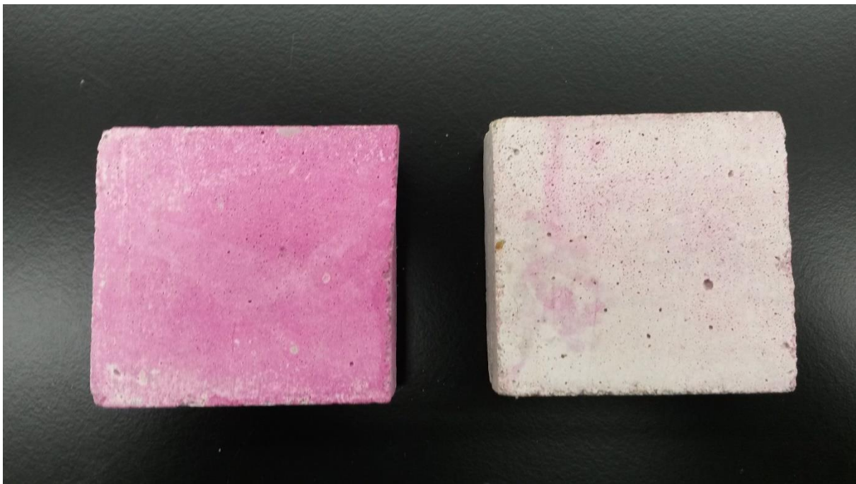
Figure 3-9 Side-by-side image of surfaces of non-carbonated (left) and carbonated (right) White TiO 2 , 0% SCM mortar specimens after treatment with phenolphthalein
