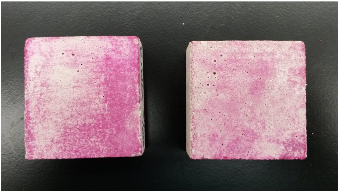
Figure 3-11 Side-by-side image of surfaces of non-carbonated (left) and carbonated (right) White \text{TiO}_2 , 30% Fly Ash mortar specimens after treatment with phenolphthalein
