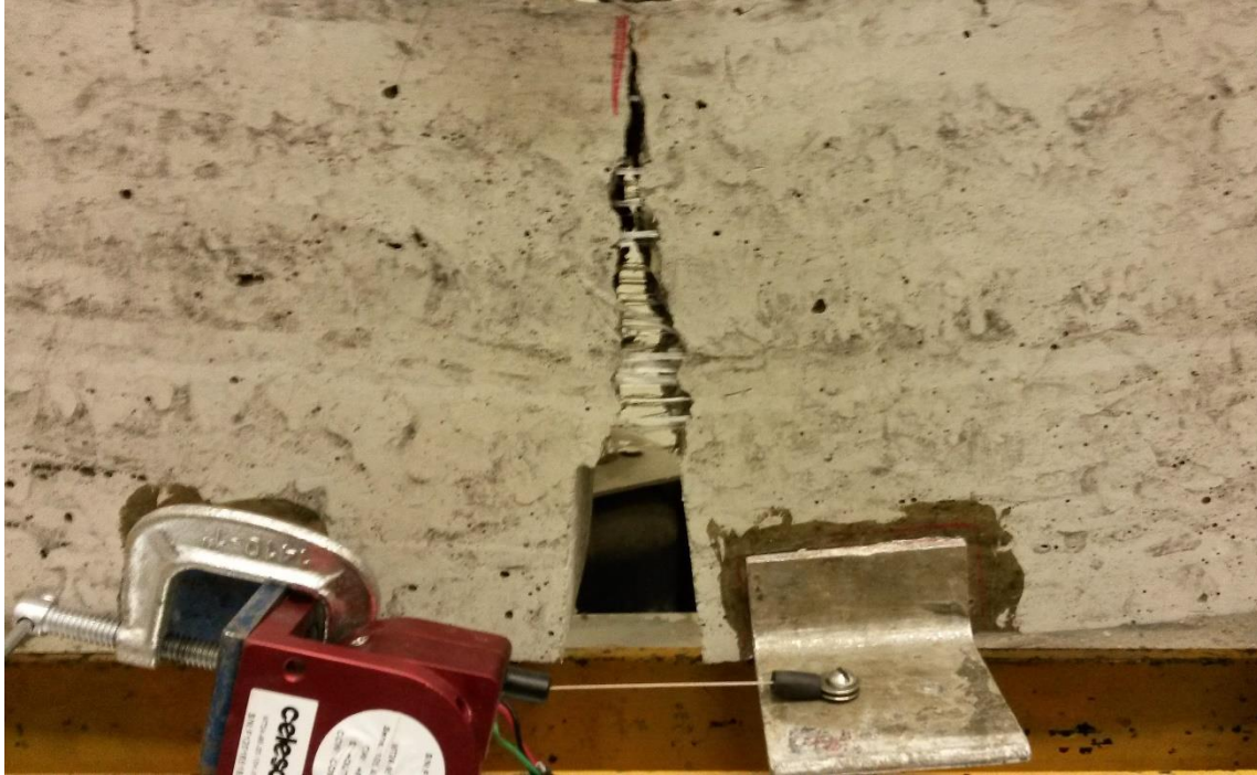
Figure 2-6 Fibers bridging the crack in a single edge notched beam specimen
