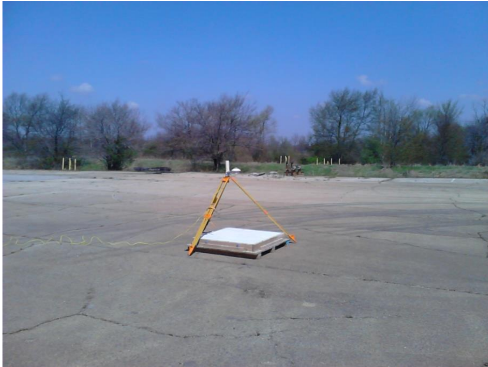
Figure 6-8 Stage II measurement of albedo over the TiO 2 concrete slab with asphalt pavement background surface
