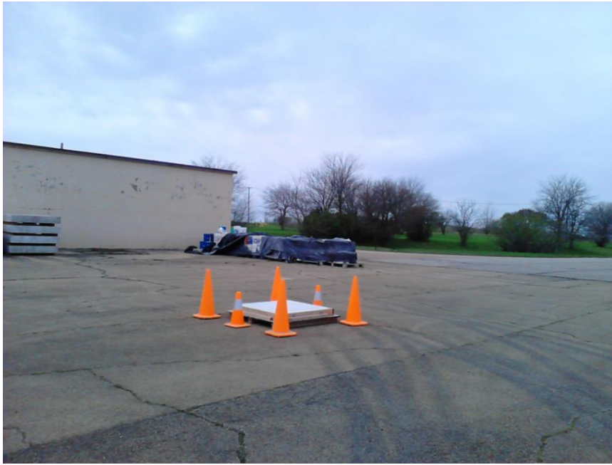
Figure 6-2 TiO 2 concrete slab on the site for stage II testing
