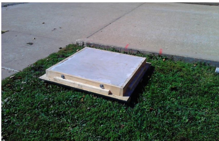
Figure 6-1 TiO 2 concrete slab on the site for stage I testing
