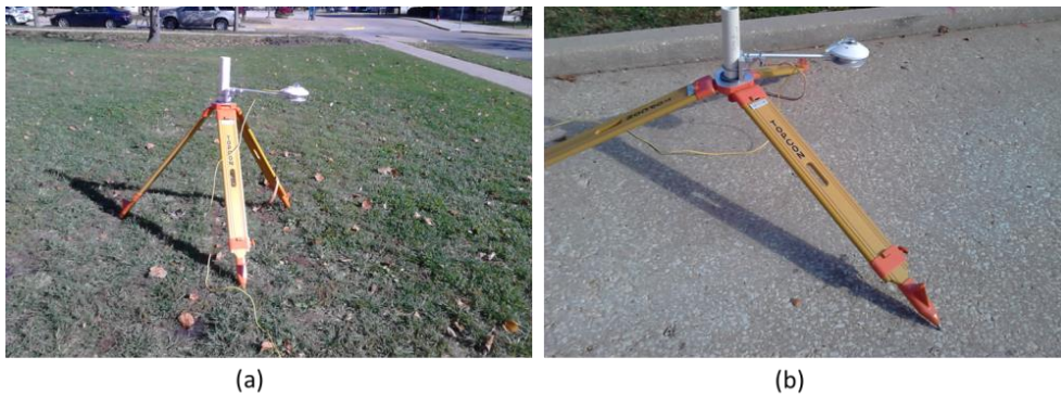
Figure 6-7 Measurement of albedo over (a) grass surface and (b) concrete ramp surface. An average of these two is called a composite 'infinite' background albedo
