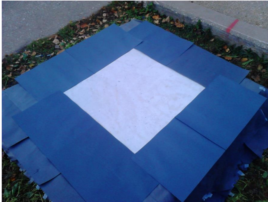
Figure 6-6 Slab covered with the 'finite background' (black paper) with an exposed size of 0.6 m
