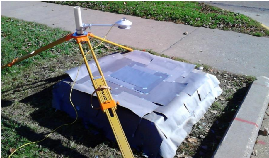
Figure 6-5 Albedo being measured at a height of 0.50 m when the exposed slab size is 0.0 m i.e., when it is fully covered in the ‘finite background’ (black paper)
