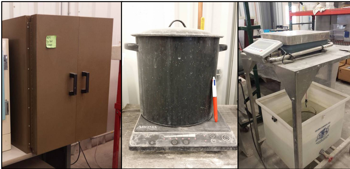
Figure 2-10: Absorption Equipment; Oven, Boiling Pot, and Balance with Buoyancy Basket
