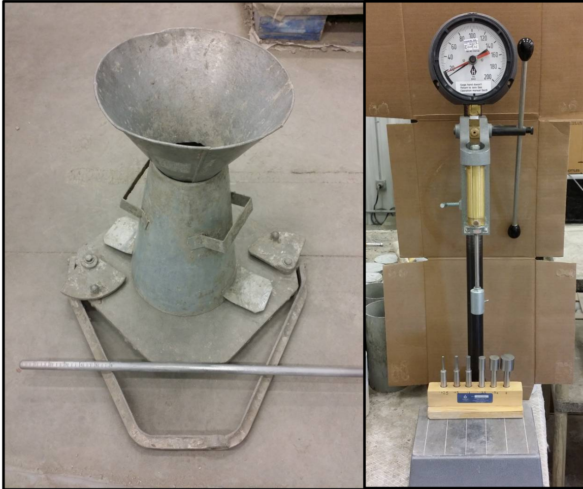
Figure 2-4: (Left) Abrams Slump Cone; (Right) Acme Penetrometer
