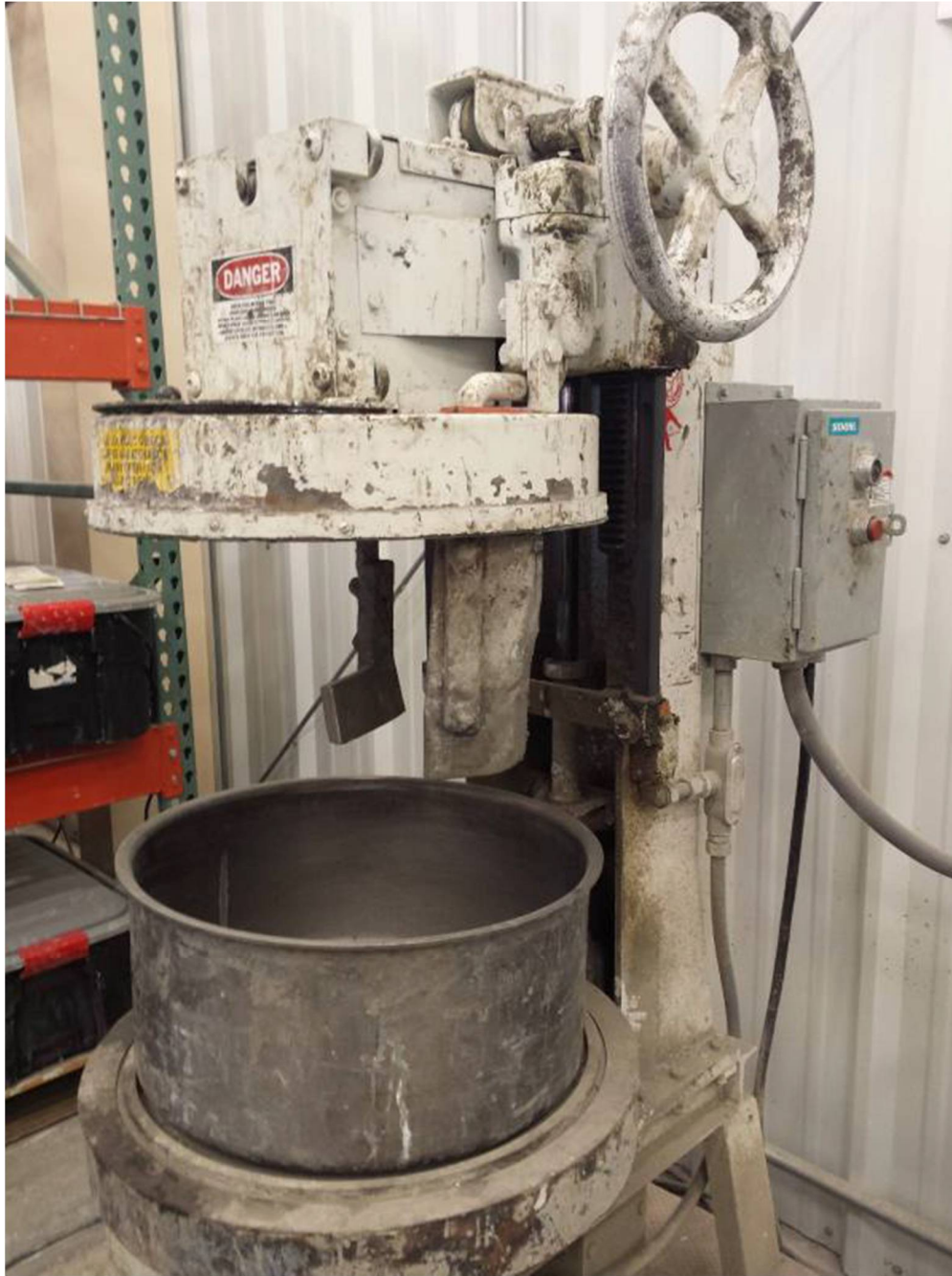
Figure 2-2: Rotating Pan Mixer
