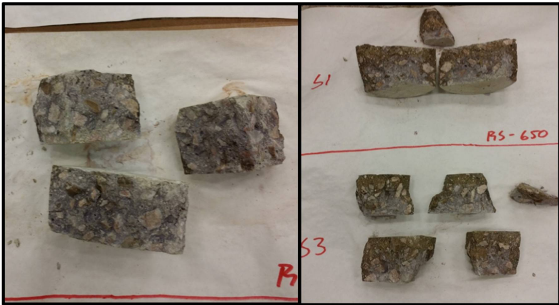
Figure 6-6: Rapid Set HES Concrete Samples Subjected to Rapid Chloride Migration Test (After Spraying Silver Nitrate)
