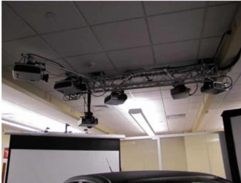
Figure 3.2 – Projectors responsible for producing the driving environment [42].
